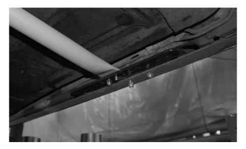
Mount the frame brackets to the frame through the original crossmember mounting holes. Then put the crossmember on top of the bracket.
