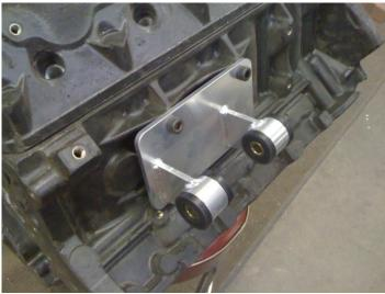
(Detailed view of driver's side motor mount on engine)
