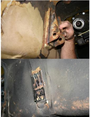
**Step2:** Position the transmission crossmember in the tunnel where the original crossmember tabs were removed, lining up the crossmember with the back edge of the original crossmember tabs. Mark the holes through the crossmember on the underside of the tunnel.
