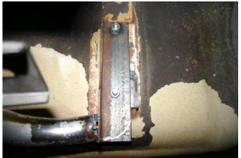
**Step 3:** Drill the holes with a <sup>1</sup>/<sub>4</sub>" drill bit all the way through both layers of the tunnel floor (make sure the carpet is removed prior to drilling). Using the <sup>1</sup>/<sub>4</sub>" holes as a guide drill through the TOP layer of the floor from inside the vehicle using a 1" holesaw (DO NOT DRILL ALL THE WAY THROUGH BOTH LAYERS OF THE FLOOR). Using a 25/64" drill bit drill through the remaining <sup>1</sup>/<sub>4</sub>" hole.
