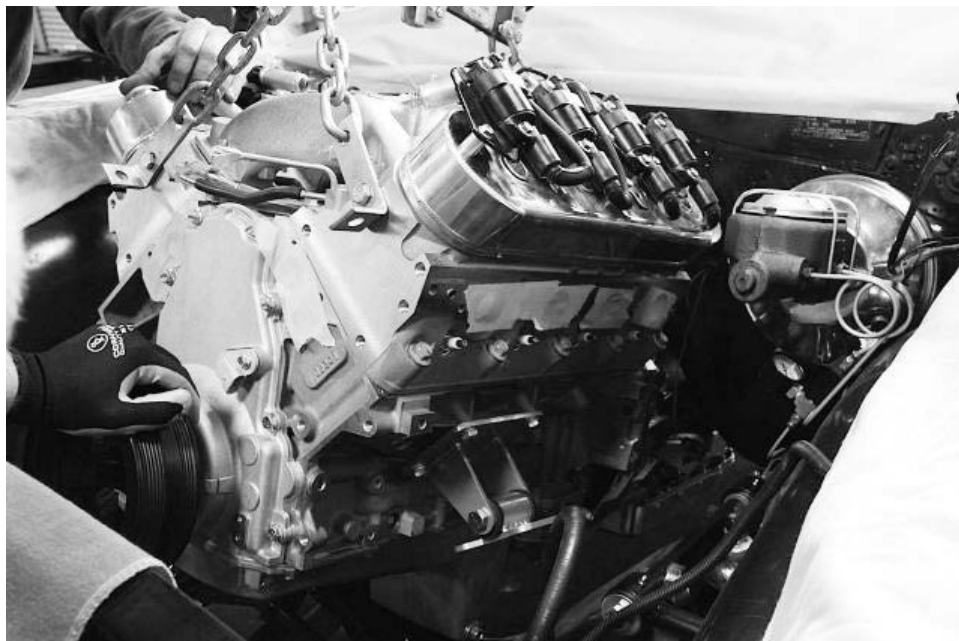
Loosely mount the engine mounts and frame mounts on the engine prior to installation.
