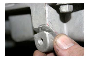
**Step 3:** Locate the motor mounts and loosely bolt them to the engine using the supplied 10mm allen head bolts. Now loosely bolt the Driver's Side (LEFT) and Passenger's Side (RIGHT) frame brackets to the engine mounts using the supplied  $\frac{1}{2}$ "-13 x 4" long bolts and nylon lock nuts. (The bolts will be tightened after the engine is set in place and everything is lined-up)
