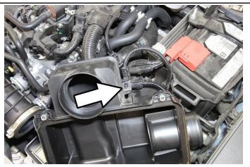
5. Flip over the upper air box assembly to access the mass air flow sensor harness clip and disconnect it from the air box. Remove the upper air box assembly from the vehicle.
