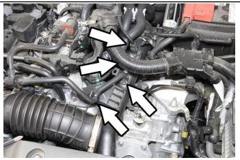
7. Disconnect the breather hose using a pair of pliers to loosen the retaining clamp. Disconnect the two harness clips from both sensors.
