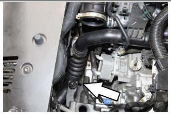
9. Loosen the hose clamp securing the hump hose from the lower charge pipe extension pipe.
