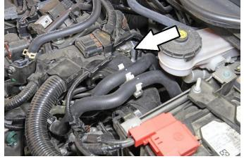
11. Loosen the hose clamp securing the throttle body hose from the throttle body and remove the factory 90-degree hose from the vehicle.
