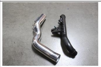
16. Remove the and secure the two sensors onto the HPS charge pipe using the provided M5x14mm bolts.
