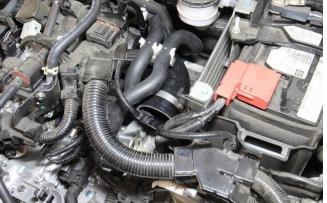
13. Insert the 90-degree hose along with the provided EMSC clamps onto the throttle body.
