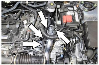
17. Insert the HPS charge pipe into the vehicle. Adjust the charge pipe into position and secure the bracket to the charge pipe using the provided M6x12mm bolt and washer. Reconnect and secure the breather hose using our provided FIC clamp to the breather barb. Reconnect the harness connectors back onto the sensors.
