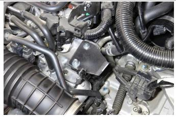
15. Insert the bracket onto the vibration mounts using the provided M6 nuts. \* Do not fully fasten the M6 nuts at this time. The bracket will need to be adjusted when installing the HPS charge pipe.
