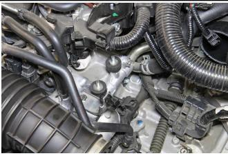
14. Install and secure the two  $\frac{1}{2}$  vibration mounts onto the factory charge pipe bracket mounts.
