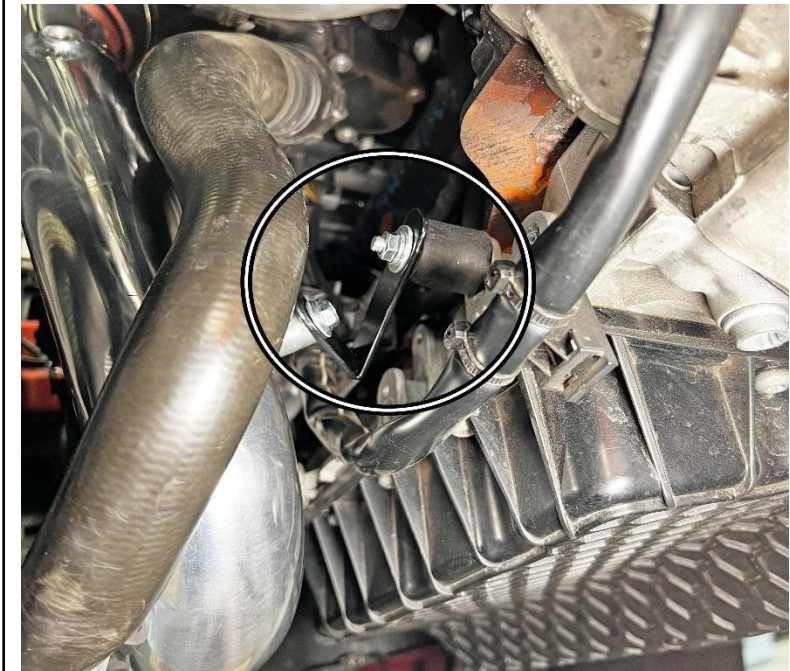
15. Install the provided 1" vibration mount into the factory cold side charge pipe mounting hole towards the center of the vehicle. Secure the "V" bracket between the vibration mount and the charge pipe using the provided M6x12 bolt, nut, and washers.
