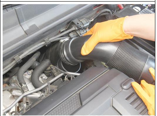
4. Remove the stock intake tube from the engine bay.
