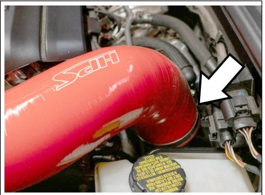
5. With the provided clamps loosely fitted on the HPS intake tube, carefully attach the turbo side first.
