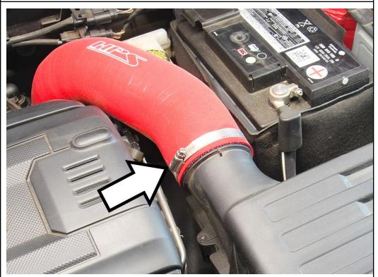
6. Connect the opposite side onto the factory air box and secure the hose clamps.
