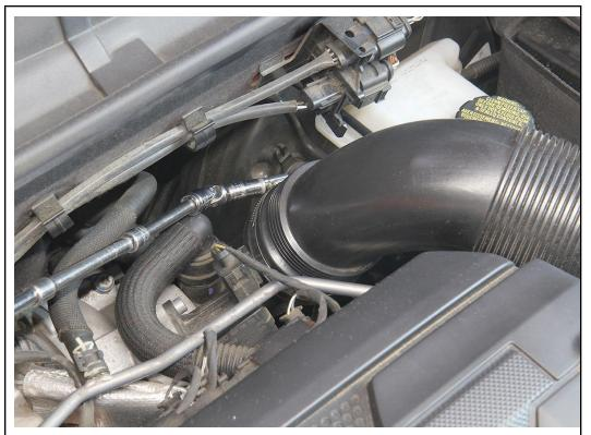
3. Loosen the hose clamp on the turbo.
