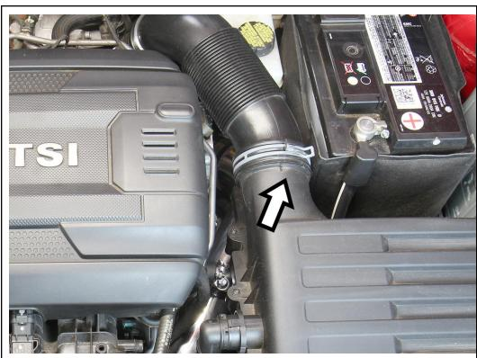
2. Pinch the ears on the clamp to loosen and disconnect the stock intake tube from the air box.
