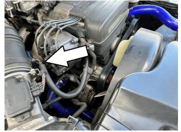
3. Disconnect the vacuum hose located on the barb near the distributor.
