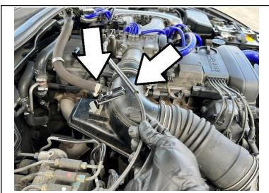
2. Disconnect the cruise control cable from the bracket. Disconnect the breather hose from the intake tube.
