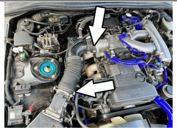
5. Loosen the hose clamps securing the intake tube from the throttle body and the MAF sensor housing. Remove the intake tube from the vehicle.
