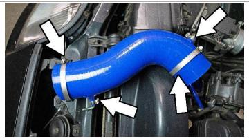
6. Secure the barbs on the HPS intake tube using the provided FIC-12 clamp and EMSC-16-27 clamp. Insert the two EMSC-70-90 clamps onto the ends of the HPS intake hose.
