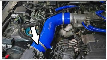
7. Insert and secure the HPS intake tube onto the MAF sensor housing first, then onto the throttle body. Re-insert the vacuum hose and the breather hose onto the HPS intake barbs.
