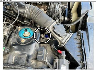
4. Remove the 10mm bolt securing the mass air flow sensor bracket to the chassis.
