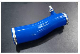
7. Install the provided hose clamps onto the HPS silicone intake tube. Tighten the clamp on the breather nipple to secure the barbed fitting.
