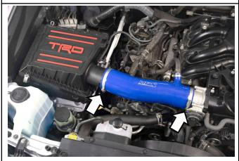
8. Insert the HPS intake onto the air box side first then onto the throttle body side and clip the air box back into place. Adjust the intake tube to the desired position and secure the hose clamps.
