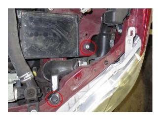
6. Once the battery is out of the way, remove the intake resonator tube by removing the 6mm bolt and unclip the plastic clip with a flat-head (blade) screwdriver.
