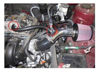
9. Install the breather hose and secure it using the 5/8" clamps provided. Reinstall the battery & engine cover.
