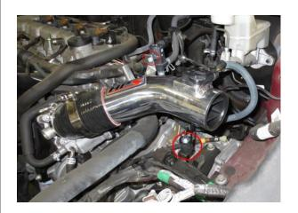
8. Install the coupler and intake pipe onto the throttle body, and secure the sensor (circled at top) using the oem bolt on to the intake pipe. Install the rubber mount and bracket to the chassis. Insert the air straighter and attach the HPS filter.
