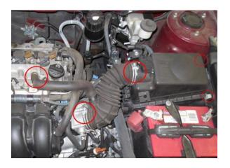
4. Remove the breather hose from the valve cover. Loosen the clamps on the factory intake hose. Unlatch the two clips that hold the top half of the intake air box and remove completely.
