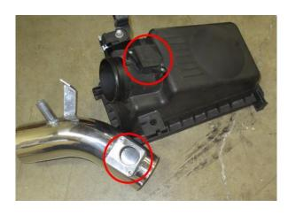
7. Install the MAF sensor onto the HPS intake pipe and secure it with the provided 4mm Allen Head bolts.
