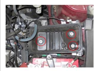
5. To remove the lower half of the air box, loosen the three screws using a 10mm wrench and remove the battery using the same tools.
