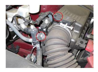
3. Unscrew the sensor attached to the factory intake tube and disconnect the mass air flow (MAF) sensor plug.
