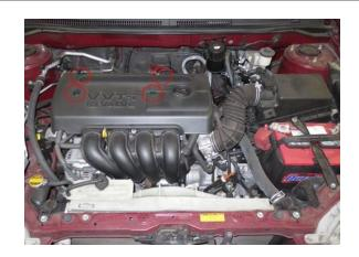
2. Remove the engine cover using a 10mm wrench.
