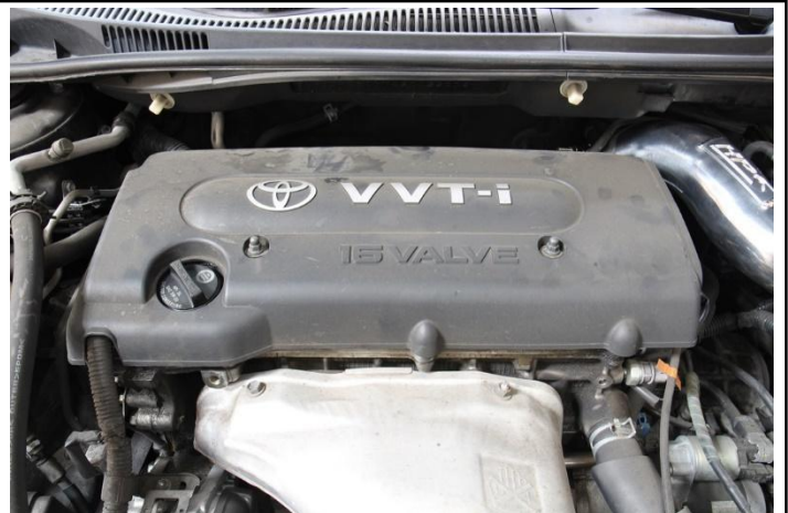
30. Re-install the engine cover back onto the vehicle.
