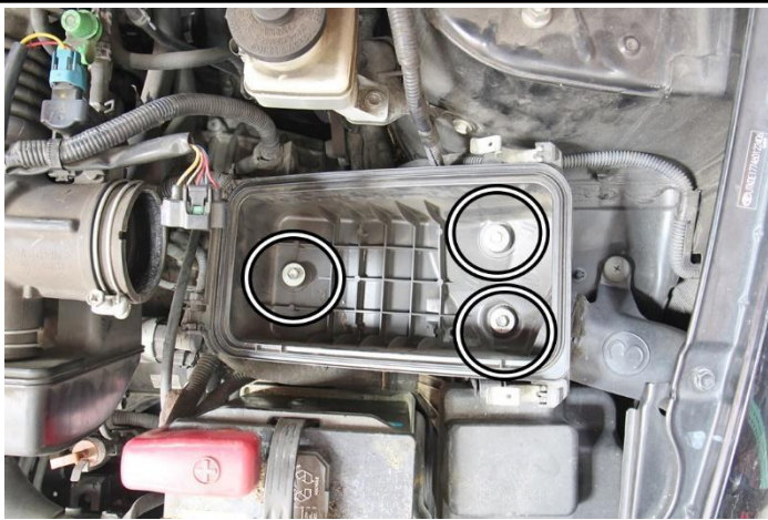
6. Remove the three 10mm bolts securing the lower air box assembly.
