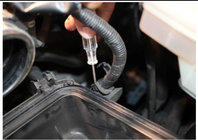
10. Unclip the MAF harness from the lower air box and remove the lower air box from the vehicle. Use a pick or a small flat screwdriver to release the clip.
