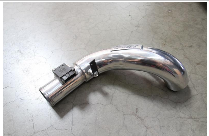
24. Remove the MAF sensor from the factory air box and install the MAF sensor onto the intake pipe using the provided Allen bolts.
