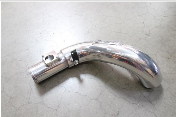
23. Install and secure the sensor bracket onto the intake using a washer and M6 bolt.
