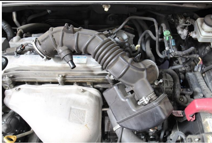
15. Remove the intake tube from the vehicle.
