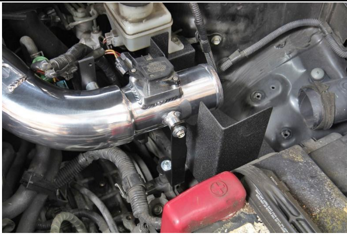
25. Insert the intake pipe into the coupler and secure the intake pipe onto the intake bracket. Once, the intake pipe is in its proper position, you can tighten the T-bolt clamp securing the pipe to the coupler.
