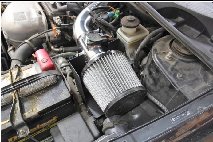
29. Install the provided HPS performance air filter.
