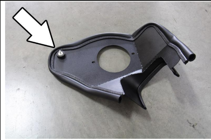
18. Install and secure the vibration mount using a washer and nut onto the heatshield.
