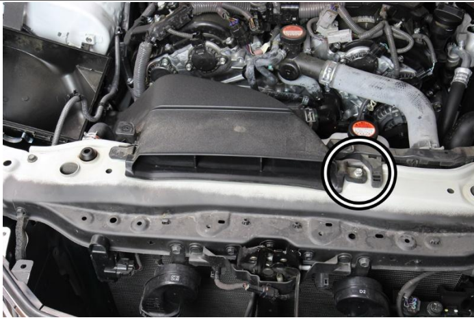
12. Remove the 10mm bolt securing the factory air duct and remove the air duct from the vehicle.
