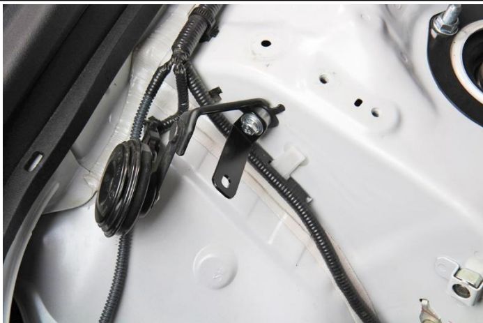
16. Install the M6 x 6mm thick .0 between the Heatshield bracket onto the air horn mounting hole. Secure the bracket using the M6 x 20mm bolt and washer provided in the hardware kit.
