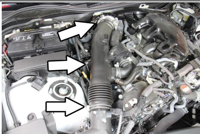
4. Loosen the hose clamps securing the intake tube from the air box and the throttle body. Then, disconnect the hose clip attached to the intake tube.
