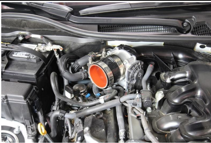
14. Install the reducer coupler along with the provided T-bolt clamps onto the throttle body.
