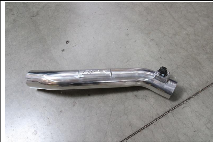
20. Install the factory mass air flow sensor onto the HPS intake. Secure the sensor using the provided M4 x 8mm bolts.
