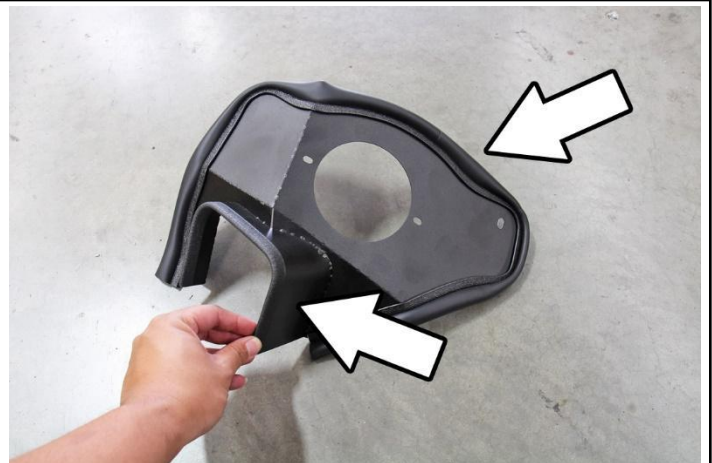
17. Install the thin edge trim onto the air duct opening of the heatshield and the bubble edge trim onto the outer edge of the heatshield.
