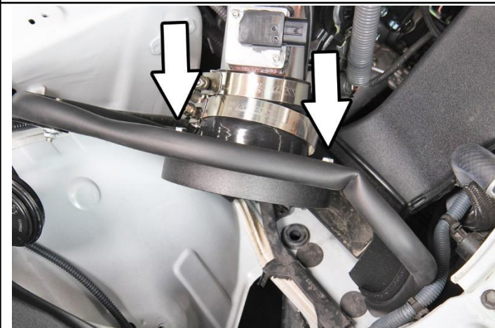
22. Insert the velocity stack into the intake coupler and secure the velocity stack to the heatshield with the provided M6 x 12mm bolts and washers. Position the intake pipe to the proper position and tighten all the t-bolt clamps securing the intake pipe to the couplers.
