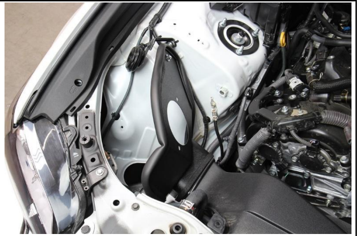
19. Re-install the factory air duct into the vehicle. Then insert the HPS heatshield and secure the vibration mount to the heatshield bracket.
