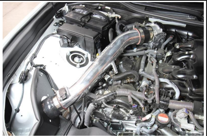
21. Install the remaining reducer coupler onto the other end of the HPS intake pipe and insert the intake pipe into the throttle body coupler.
