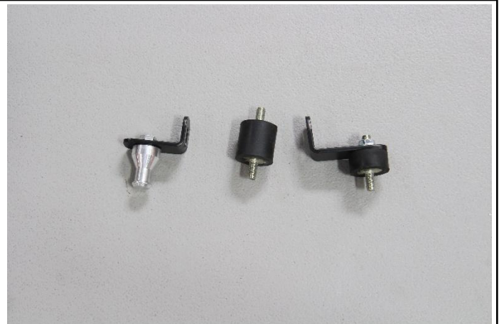
11. Install and secure the smaller "L" bracket onto the provided M6 bung using a M6x12 bolt and washer. Loosely install the larger "L" bracket onto the 1/2" vibration mount using a nut and washer.
