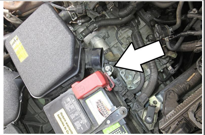
13. Insert the 1" vibration mount into the factory air box mount near the air duct.
