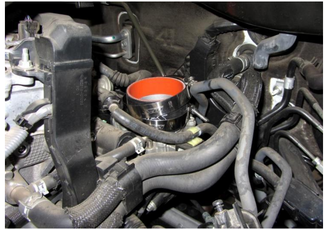
9. Install the HPS coupler onto the throttle body along with the provided T-bolt clamps.
