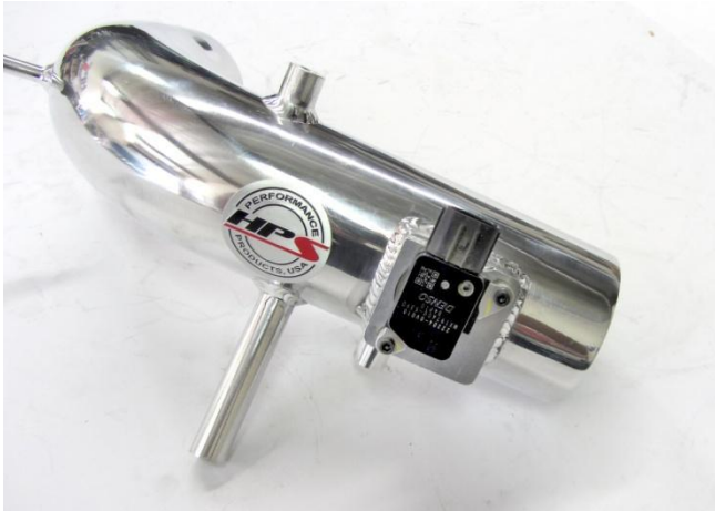
14. Remove the MAF sensor from the stock air box and transfer it over to the HPS intake pipe. Use the included 4mm Allen bolts to secure it to the pipe.
