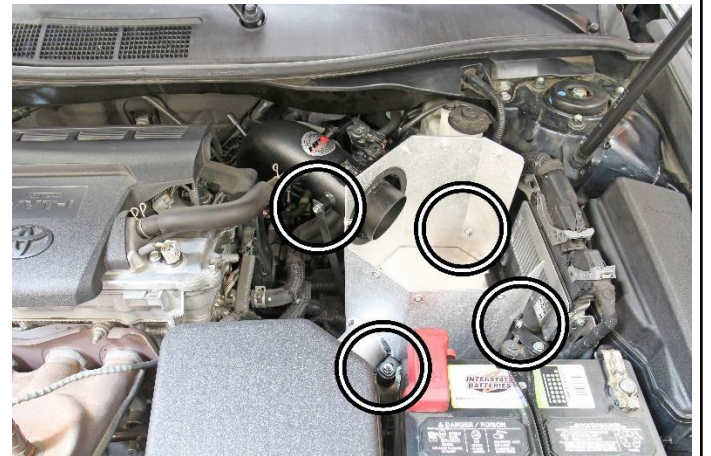
21. Insert the heat shield into the vehicle, then secure all the brackets to the heat shield using the provided M6x12mm bolts, nuts, and washers. Adjust the HPS intake pipe into position and secure the intake pipe to the bracket.
