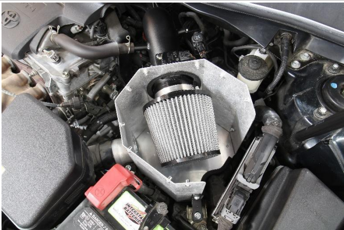
22. Install the provided HPS performance air filter.
