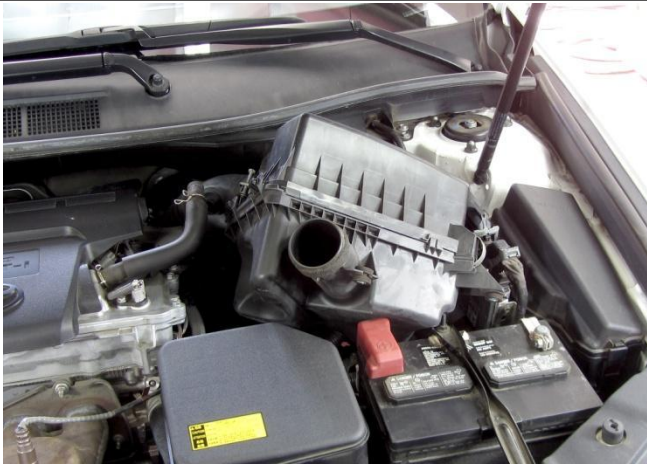
6. Remove the air box from the engine bay.
