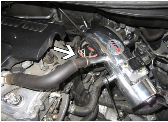
18. Insert the factory breather hose onto the HPS intake barbs.
