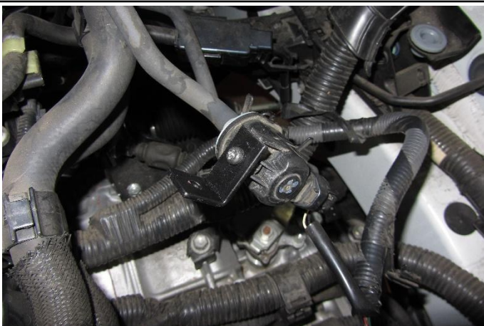
16. Install and secure the "L" bracket onto the EVAP valve by reusing the factory screw.
