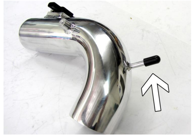
15. If your vehicle has an additional hose, install it onto the intake pipe. If your vehicle does not have the additional hose, use the 5/16" vacuum cap included in the kit to block it off.
