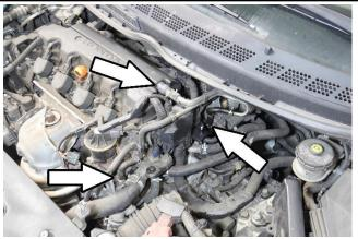
8. Loosen the hose clamps securing the breather hose from the valve cover. Using a pair of pliers, loosen the factory coolant hose clamps securing the coolant hose from the throttle body and the lower hose assembly.
