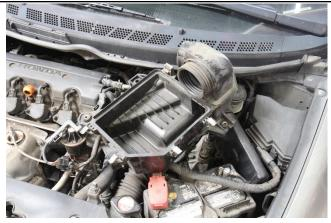
6. Lift the lower air box assembly from the rubber grommet and remove the lower air box assembly from the vehicle.
