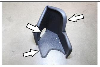
14. Install the provided bubble edge trim and thin edge trim in the areas shown above. Be sure to cut any excess lengths.
