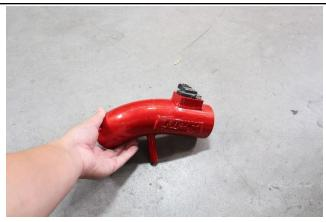
19. Remove the mass air flow sensor from the factory air box. Insert and secure the MAF sensor using the provided M4x8mm allen bolts.
