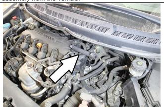
10. Install and secure the 16mm EPDM hose along with the provided EMSC clamps onto the breather barb.
