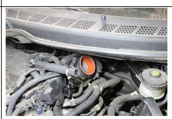
11. Insert the reducer coupler along with the provided T-bolt clamps onto the throttle body.
