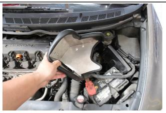
16. Insert the heatshield into the vehicle. Insert the factory air duct into the heatshield.
