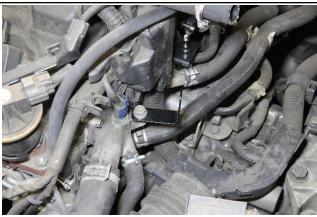
13. Loosely insert the provided "L" bracket reusing the factory bolt removed in the last step along with the 8mm washer.
