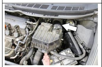
4. Disconnect the factory air intake hose from the upper air box assembly and remove it from the vehicle.
