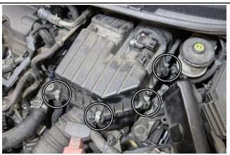
3. Disconnect the four retaining clips securing the upper air box assembly.
