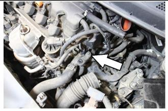
12. Remove the 10mm bolt from the factory air box bracket shown above.
