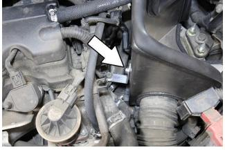
17. Secure the "L" Bracket to the heatshield using the provided M6x16mm bolt, nut and washer.
