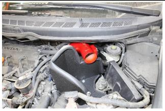
20. Insert the HPS intake pipe into the throttle body coupler. Position the intake pipe and secure the T-bolt clamp.
