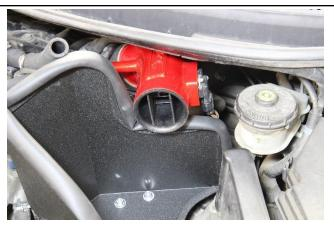
21. Insert the provided air straightener into the intake pipe. Re-connect the MAF sensor harness connector, then insert and secure the EPDM hose onto the intake pipe barb.
