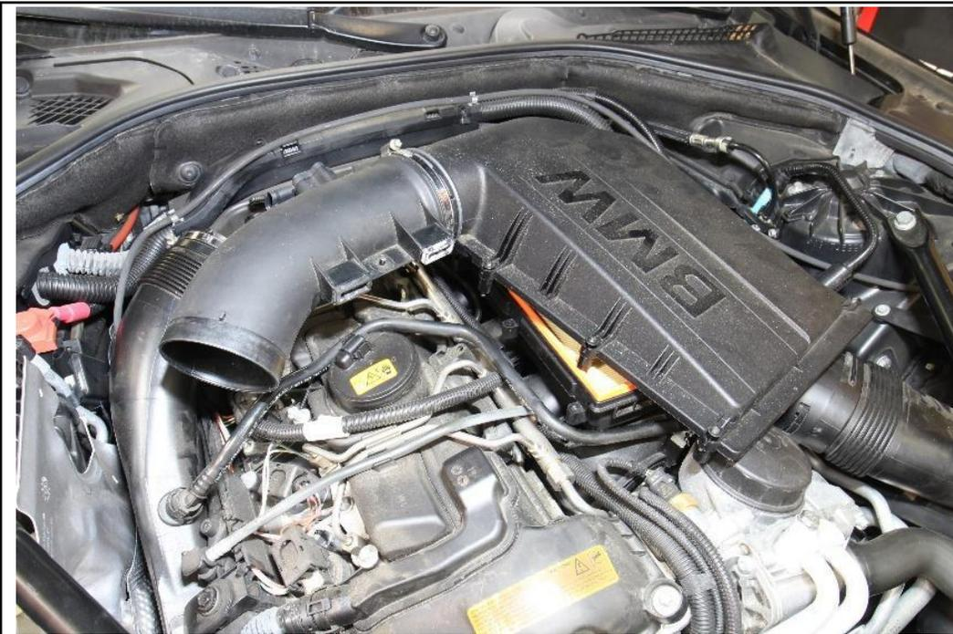
5. Remove the air intake tube along with the upper air box assembly from the vehicle.
