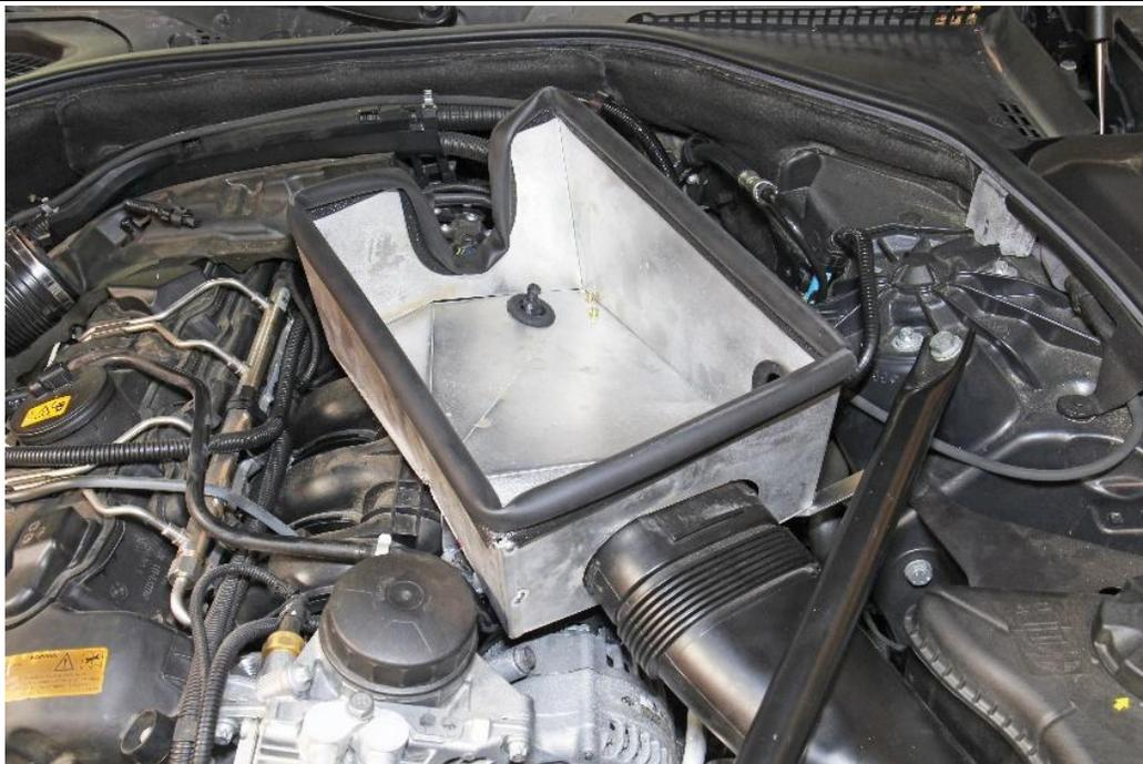
14. Insert the heat shield into the vehicle.
