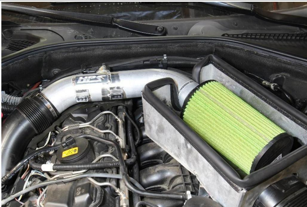
18. Insert and secure the HPS intake pipe onto the vehicle. Reconnect the MAF sensor harness connector.
