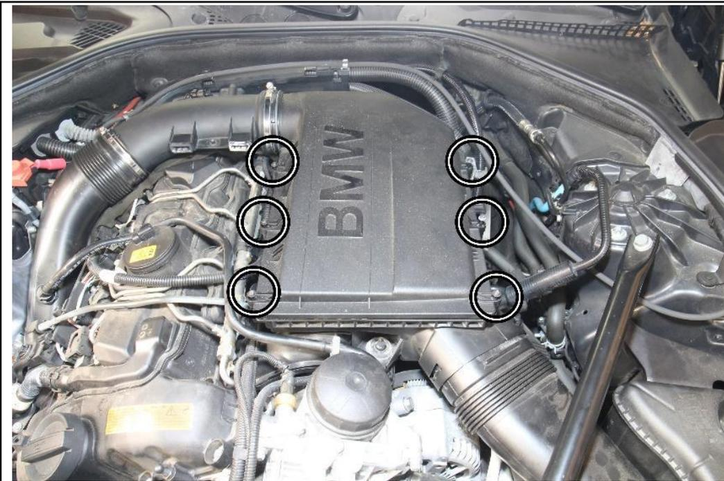
3. Loosen the six Torx bolts securing the upper air box assembly.
