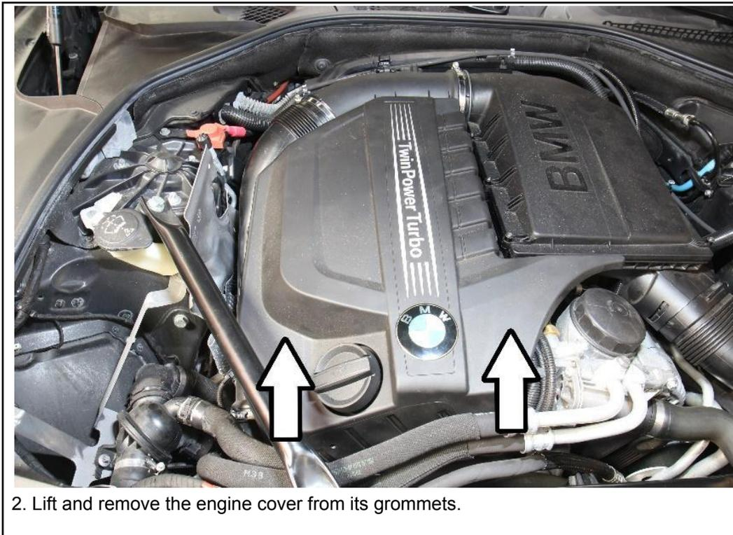
2. Lift and remove the engine cover from its grommets.
