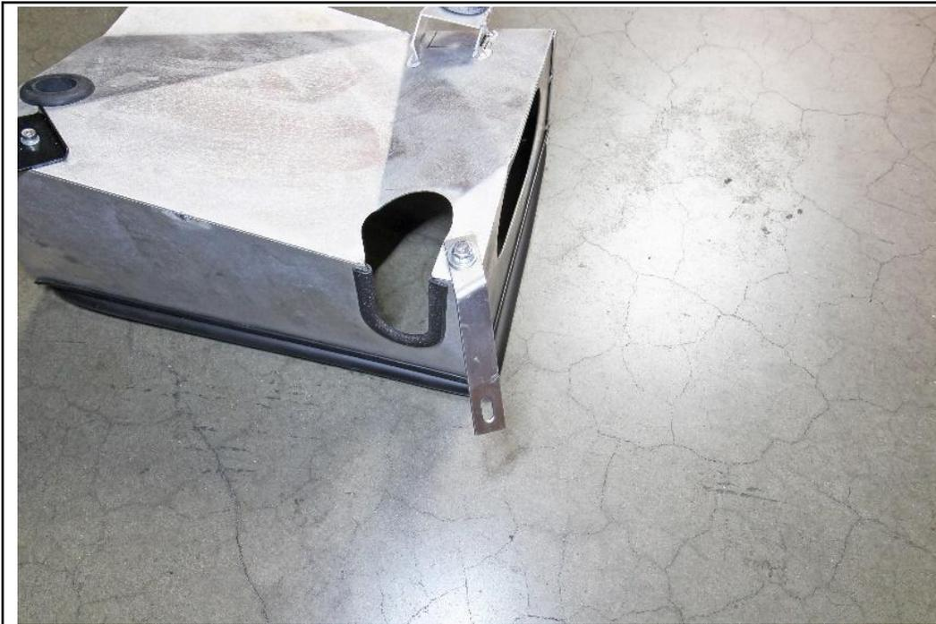
11. Loosely install the provided heat shield bracket onto the heat shield using the M6x16mm bolt, nut, and washers.
