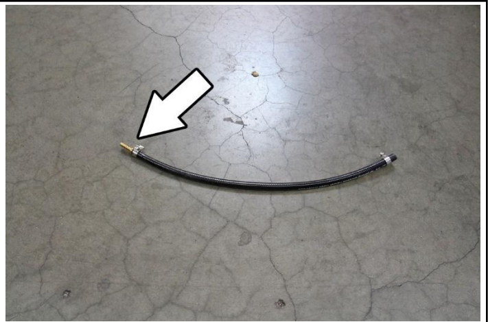
13. Insert the provided 5/16" barb fitting into the 1/4" heater hose and secure the hose using a FIC-11 clamp.
