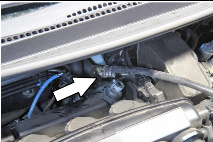
14. Using another FIC-11 clamp, insert the clamp onto the factory coolant hose. Insert and secure the other end of the 5/16" barb into the factory hose.
