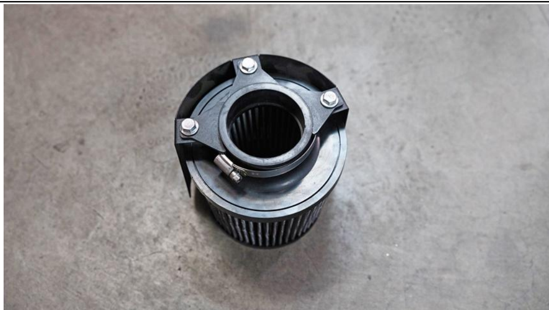
32. Use the provided EMSC-70-90 clamp to secure the heat shield onto the HPS performance air filter.
