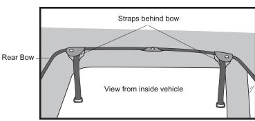
Make sure that the straps sewn into the rear of the top are behind the rear bow.
