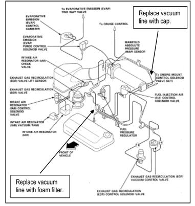
equipped with one, a vacuum line will run from the FIA control valve to the air intake pipe. During installation of the AEM<sup>®</sup> intake system, this vacuum line should be removed. Install a vacuum foam filter onto the exposed nipple of the FIA control valve.
