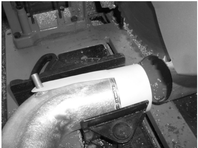
i) Saw your pipe at the edge of the template.
