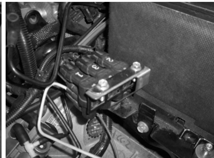
b) Retain the vacuum assembly bracket.
