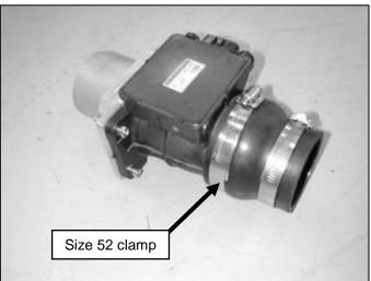
c. Attach the rubber reducer to the MAF sensor using the size 52 hose clamp.
