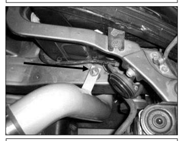
i. Install rubber mount into frame and attach the lower intake pipe's support bracket as shown. Secure with a lock nut and fender washer but do not completely tighten the lock nut. See the diagram below for proper installation of the rubber mount.
