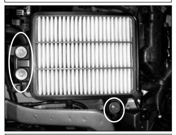
f. Loosen the three bolts securing the air box in place. Remove air box and snorkel from vehicle.
