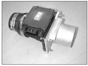
b. Attach the MAF adapter to the MAF sensor using the supplied bolts and lock nuts.
