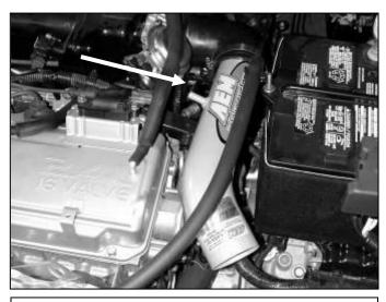
e. Insert the upper intake pipe into the rubber elbow. Ensure the nipple on the intake pipe is pointing toward the center of the vehicle as shown.
