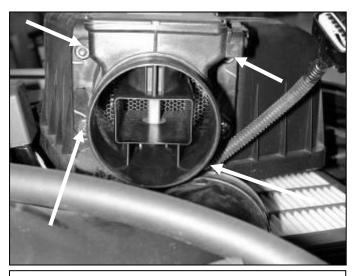
d. Loosen the four nuts that secure the MAF sensor to the air box. Carefully remove and set aside the MAF sensor.
