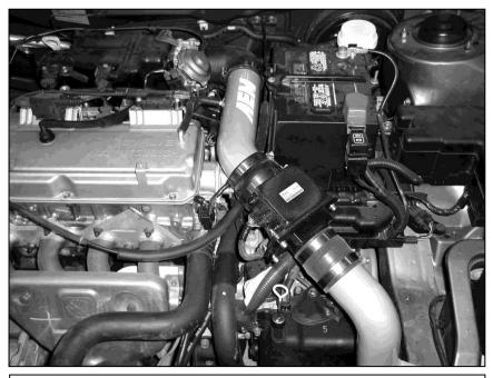
k. Install the AEM<sup>®</sup> air filter onto the lower end of the intake pipe. Check the clearance of the air filter and tighten the hose clamp once proper fitment is achieved.
