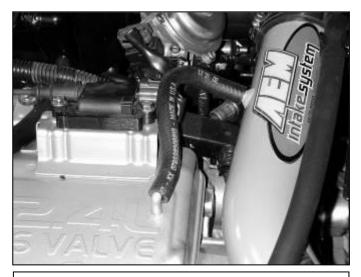
f. Install the supplied breather hose as shown. Secure both ends with supplied <sup>3</sup>/<sub>4</sub>" hose clamps.
