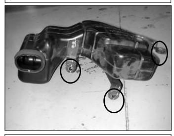
h. Loosen the three bolts that secure the lower air box and remove from the vehicle.
