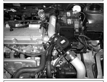
h. Plug the wiring harness into the MAF sensor and attach the lower intake pipe to MAF sensor using the provided silicone hose and two hose clamps.
