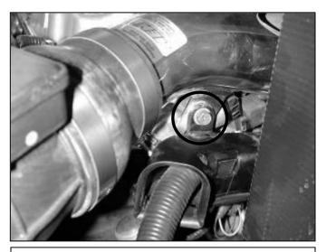
g. Attach the bracket on the upper pipe to the engine using the supplied 6mm bolt and washer. Place the pipe's tab behind the stock plastic tab. Attach the MAF sensor assembly to the intake pipe as shown.
