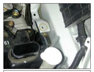
k. Locate the bolt securing the lower resonator in the engine compartment and remove it.
