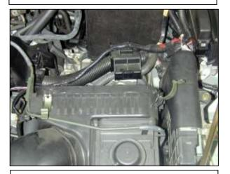
g. Unclip the air filter housing lid and remove the lid and the air filter.
