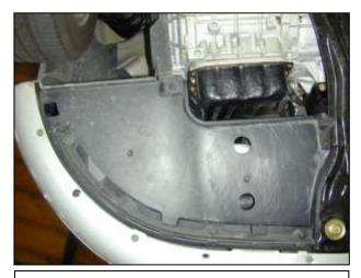
I. Remove the five screws and four plastic connectors securing the driver's side underbody splash shield to the chassis.
