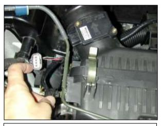
f. Unclip the Mass Air Flow (MAF) sensor wiring harness from the air filter housing. These clips can be removed undamaged from the harness using a small flat head screwdriver. Unplug the MAF sensor from the engine harness.
