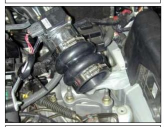
j. Install the supplied hump hose on to the end of the lower intake pipe. Secure using a #44 hose clamp.
