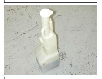
m. Unplug the radiator fan harness. Unhook the radiator overflow hose from the reservoir and remove the reservoir.
