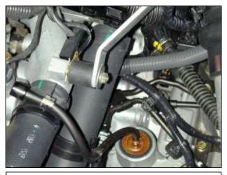
f. Align the intake mounting bracket with the previously installed rubber mount and secure using a 6mm flat washer and serrated nut.
