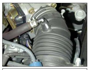
c. Remove the breather hose from inlet air hose by compressing the spring clamp and pulling it off.
