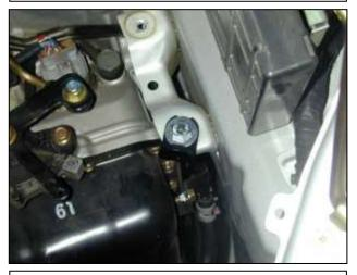
i. Install the lower pipe bolt on mounting bracket using the supplied M8 bolt and washer as shown. Leave this bracket fairly loose.
