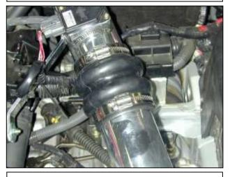
k. Slide the lower intake pipe in from the bottom and align the upper and lower pipes. Slide the hump hose over the end of the upper intake pipe and secure using a #44 hose clamp.
