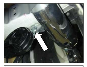
I. Align the fixed lower intake pipe bracket with the hole where the horn was previously removed. Install the supplied M8 bolt, washer, and horn.
