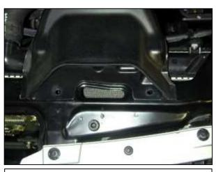
b. Remove the two plastic rivets holding the intake duct to the radiator support.
