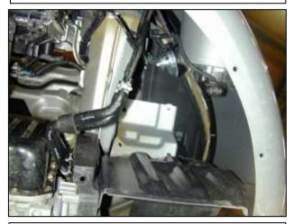
n. Remove the bolt securing the horn to the chassis and remove the horn. Remove the remaining two bolts securing the lower resonator to the chassis and remove the resonator.
