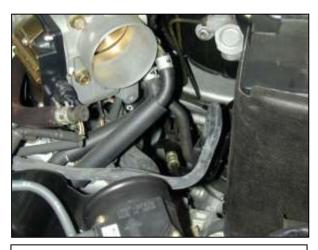
e. Loosen the hose clamp on the air filter housing and remove the air inlet tube and upper resonator.
