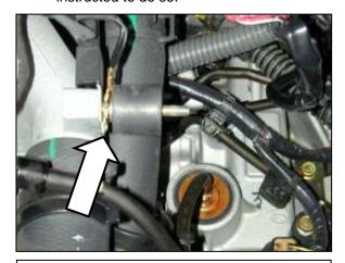
b. Install the supplied rubber mount where the bolt was removed in step 20 using the  $\frac{1}{4}$ " flat washer as shown.
