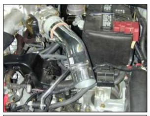
e. Check that the inside of the AEM® intake pipe is free from debris. Install the intake pipe into the previously installed coupler as shown.
