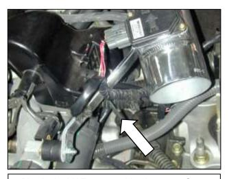
g. Plug in the MAF sensor wiring harness. Secure the plug and extra wire for the bypass solenoid using a 6" zip tie.
