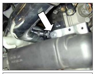
m. Install the M6 bolt into the bracket installed in step 3h. Thread the bolt into the threaded bung on the lower intake pipe. Tighten the bolts loosened in step 2i.
