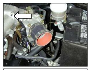
c. Install the 2.75" silicone coupler onto the throttle body and secure using a #44 hose clamp. Also, install the vacuum cap on the intake manifold nipple as indicated above.
