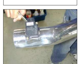
d. Install the previously removed MAF sensor into the upper intake pipe using the two bolts removed in step 2p.
