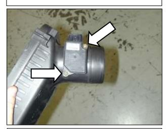
p. Remove the two bolts securing the MAF sensor to the air filter housing and remove the MAF sensor. Be careful not to damage the sensor.
