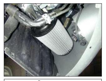
n. Install the AEM<sup>®</sup> air filter onto the end of the intake pipe. Push the air filter over the intake pipe until the stop in the air filter is reached. Then install one hose clamp to secure the filter onto the intake pipe.
