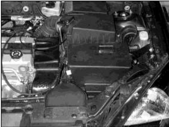
a. Factory air box system installed.
