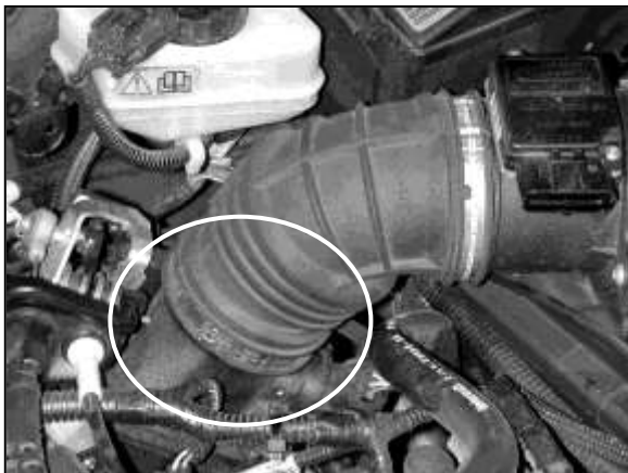
c. Remove the clamp securing the primary inlet tube to the throttle body.
