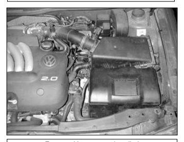
Factory airbox system installed
