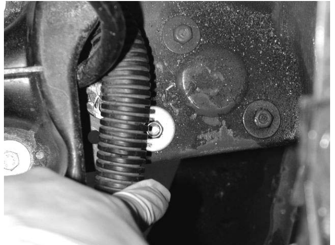
c) The rubber mount should be installed from the bottom, with the washer and Nylock nut on top.
