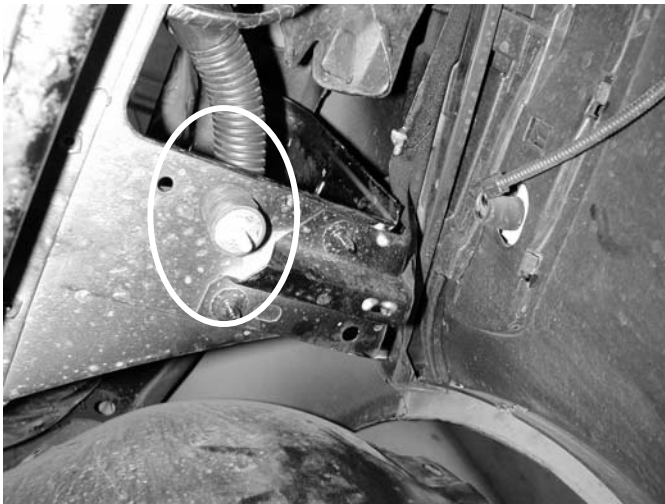
b) Using one supplied washer and one Nylock nut, install the supplied rubber mount into the hole beneath the battery tray that is towards the fender.
