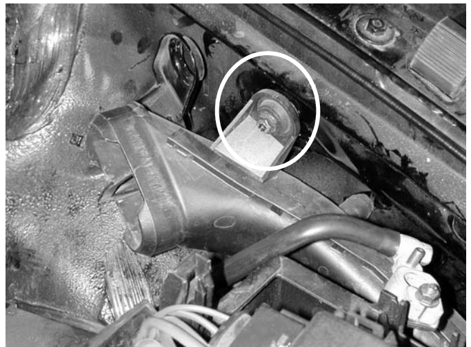
h) Remove the nut that secures the lower air duct to the fender well. Remove the lower air duct.
