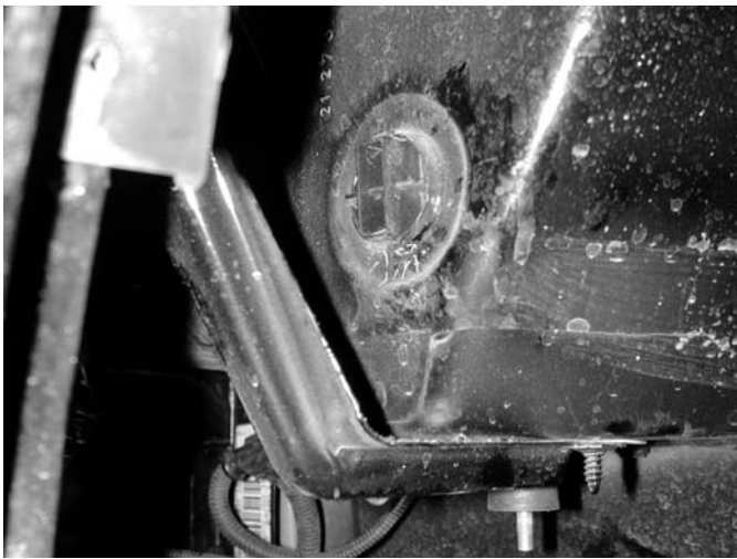
n) Squeeze the tabs on the plastic cradle that used to hold the wire harness connector in the engine bay. Remove the plastic cradle.
