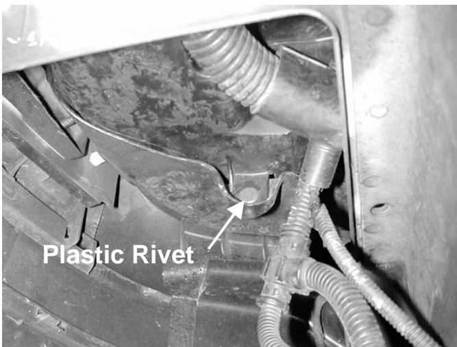
p) Remove the one plastic rivet underneath the headlight housing.
