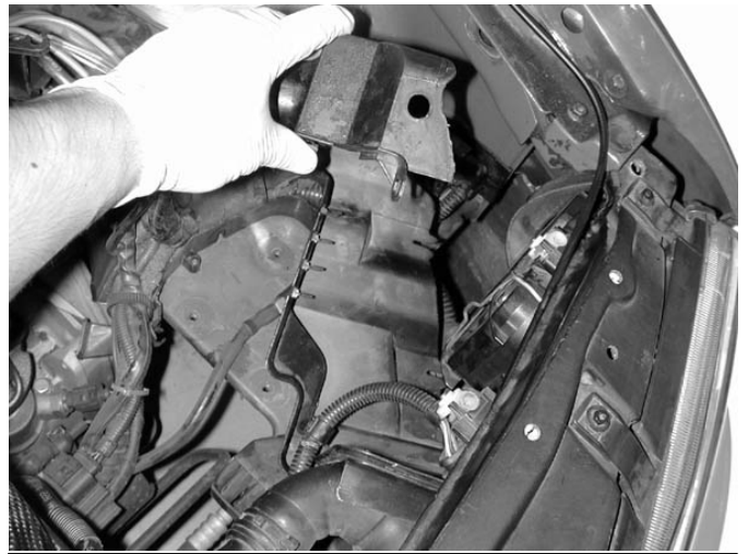
q) Pull the plastic guard from the engine bay. This piece will not be reused with the AEM inlet system.
