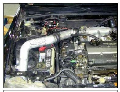
AEM® intake system installed
