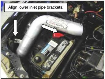
h. Insert the lower inlet pipe. Align both brackets with the rubber mounts. If the hole isn't big enough, the brackets will not align with the rubber mounts. Refer to the rubber mount assembly diagram.
