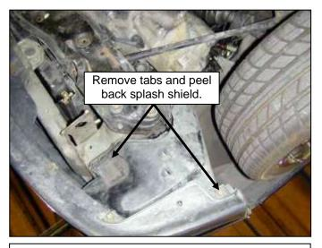
c. Remove the two tabs that secure the lower splash shield. Peel down to gain access to the cavity left by the resonator.
