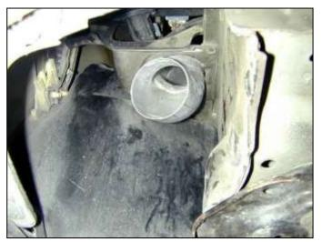
I. Make sure the lower inlet pipe clears the newly widened opening. Attach the air filter element and secure.
