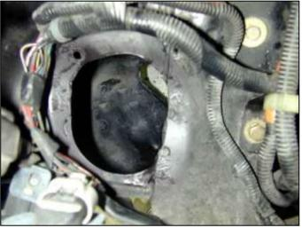
d. The cavity left by the resonator must be enlarged for clearance of the AEM® intake pipe. The lower inlet pipe is 3.00" in diameter. You will need to open up the hole to accommodate the pipe diameter. A minimum of at least 3.25" diameter is recommended. The use of a specialized power tool will be needed to cut through the inner fender so the AEM® intake pipe is able to clear the inner fender opening. Remove any burrs and line the fender opening with the rubber edge trim.
