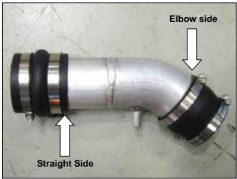
i. Assemble the upper intake pipe installation as shown. On the elbow side, attach the reducer coupler and hose clamps. On the straight side, attach the hump hose and hose clamps. Do not completely tighten.
