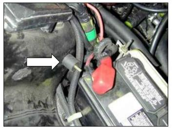
g. Insert the rubber mount and tighten.
