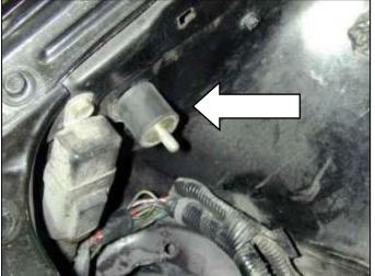
f. Insert the rubber mount and tighten.
