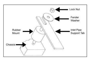
Proper installation of the rubber mount assembly.
