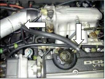
k. Attach the breather hose to the upper inlet pipe and the valve cover. Secure both ends with the provided hose clamps.
