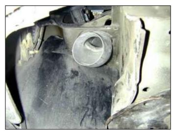
e. Ensure that any rough or sharp edges are smoothed and that the AEM® intake pipe is able to clear the opening without touching any part of the inner fender. Test fit the intake pipe to ensure there is adequate clearance.
