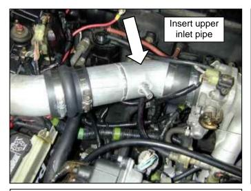
j. Attach the upper inlet pipe as shown. First attach the hump hose to the lower inlet pipe. Then attach the elbow side to the throttle body.
