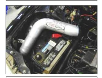
g. Insert the lower inlet pipe. Align both brackets with the rubber mounts. If the hole isn't big enough, the brackets of the inlet pipe will not align with the rubber mounts. Refer to the diagram on the next page for proper rubber mount installation.
