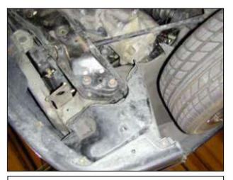
c. Remove the two tabs that secure the lower splash shield. Move the splash shield out of the way to gain access to the inner fender well where the factor resonator is located. Save the plastic tabs, they will be reused in a later step.
