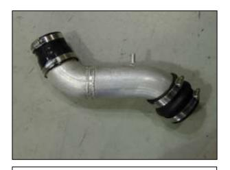
h. Assemble the upper inlet pipe as shown. On the throttle body side, attach the reducer coupler and hose clamps. On the nipple side, attach the hump hose and hose clamps. Do not completely tighten the hose clamps.
