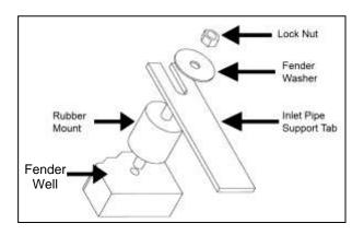
Proper installation of the rubber mount assembly.
