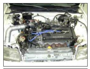
AEM® intake system installed
