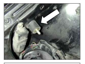
e. Insert the rubber mount in the location specified and tighten.
