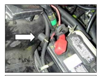
f. Insert the rubber mount in the location specified and tighten.
