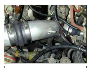
i. Install the upper inlet pipe as shown. First, attach the hump hose side of the inlet pipe onto the upper end of the lower inlet pipe. Then attach the upper end of the upper inlet pipe onto the throttle body.
