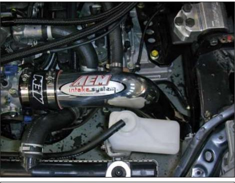
AEM<sup>®</sup> intake system installed
