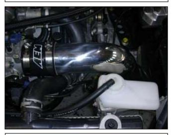
f. Insert the inlet pipe into the hose adapter and align the mounting bracket with the rubber mount installed in step #3d.
