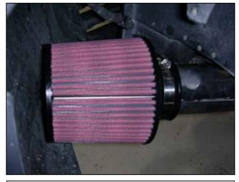
i. Install the AEM<sup>®</sup> air filter onto the end of the inlet pipe and secure in place with the supplied hose clamp.
