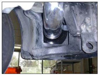
k. The fender liner must be trimmed for the intake system to fit properly. **NOTE: Failure to install the fender liner will result in diminished performance and increase the potential for engine damage due to water ingestion in rainy conditions.**
