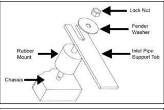
Proper installation of the rubber mount assembly.
