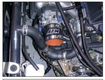
c. Install the supplied hose adapter onto the throttle body using the supplied #40 and #44 hose clamps. Use the #40 hose clamp on the throttle body.
