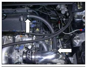
h. Attach the supplied ½" breather hose to the intake pipe's nipple; connect the opposite end to the valve cover's inlet. Secure each end of the breather hose in place with the two supplied hose clamps.
