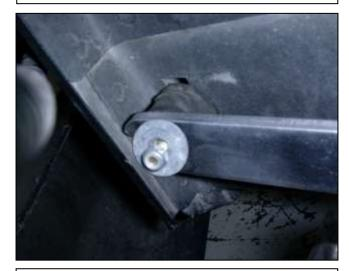
g. Slide the intake pipe's mounting bracket onto the rubber mount, and secure in place with the supplied washer and nut.
