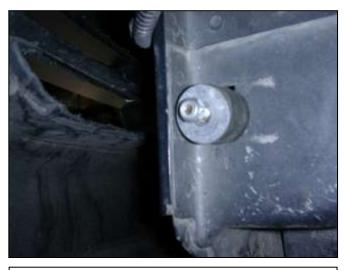
d. Locate the hole on the driver side frame rail in the front area of the vehicle. Install the supplied rubber mount into the hole as shown. Install the supplied wash and nut into the rubber mount.
