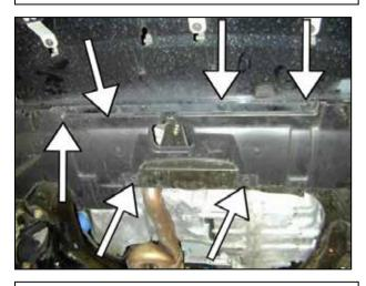
o. Remove the plastic clips. Pull the lower splash shield away from the vehicle.
