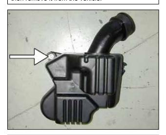
u. Remove the second bolt and remove resonator from the vehicle.
