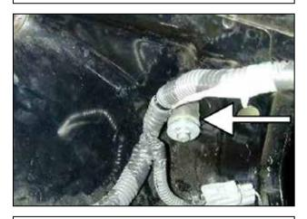
d. Insert the rubber mount stud through the hole.
