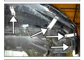
n. Remove the plastic clips and bolts.
