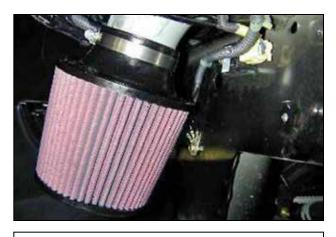
i. Install the air filter onto the end of the intake pipe.
