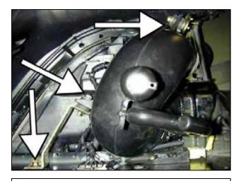
q. **Manual transmission vehicles:** The stock resonator should look similar to the image above. Remove the two mounting bolts holding it in place and the mounting bracket attached to the frame. Proceed to step 3.
