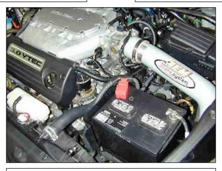
AEM® intake system installed.
