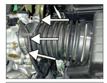
b. Remove the inlet tube by removing the hose clamp, the spring clamp and releasing the wire loom from the inlet tube's clip. Pull the breather hose off the inlet tube, then remove the inlet tube.
