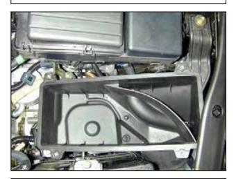
f. Remove the two bolts that hold the lower air box to the chassis. Remove the lower air box from the vehicle.
