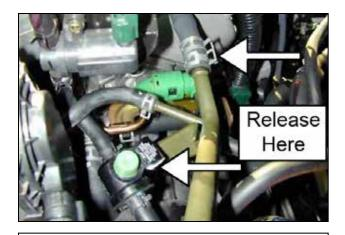
g. Release the spring clamp on the breather hose attached to the valve cover. Pull the hose off of the valve cover. Release the clip that holds the vacuum hose to the breather hose.
