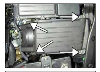
c. Loosen the four screws that secure the upper air box.
