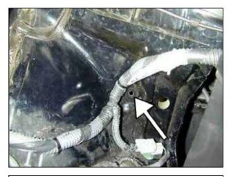
c. Release the wire loom from the hole in the fender well.
