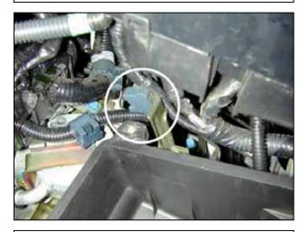
e. Remove the wire clamp from the lower air box bracket.
