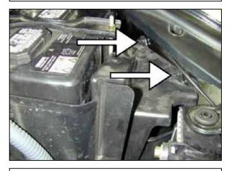
j. Remove the plastic cover by first removing the two plastic clips, then remove the plastic cover.
