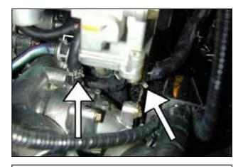
h. CAUTION: Ensure the engine is completely cool before removing the coolant hose, or hot coolant will escape from the cooling system and cause injury or damage. Be sure to capture any lost coolant in a clean container. Release the two spring clamps on the coolant feed hose attached between the throttle body and coolant source.
