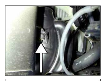
r. **Automatic transmission vehicles:** Loosen and remove the resonator bolt.
