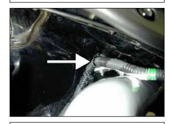
g. Place the intake support bracket behind the washer on the rubber mount as shown. Refer to the diagram on the following page for proper rubber mount assembly.
