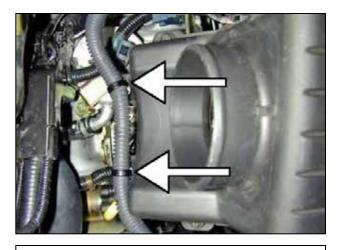
d. Carefully lift the upper air box. Pinch the bottoms of the wire ties with pliers and remove them from the upper air box. Remove the upper air box and air filter from the vehicle.
