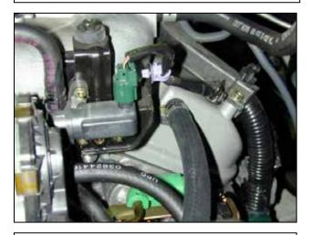
j. Install ½" ID hose over the breather nipple on valve cover. Secure it with a supplied 1" hose clamp.
