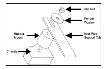
h. Proper installation of the rubber mount assembly.
