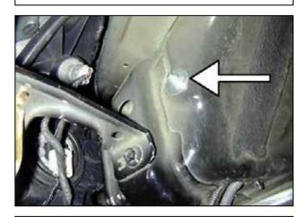
e. Secure the rubber mount stud from the inside of the fender well with the supplied washer and lock nut.
