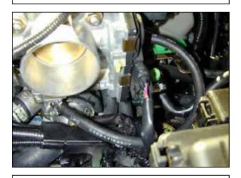
i. Remove the stock breather/coolant hose system. Route the supplied 5/16" ID hose as shown. Secure the hose to both coolant nipples with the supplied 3/4" hose clamps.
