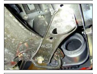
s. Pull the plastic inlet pipe from the air box and then remove it from the vehicle.
