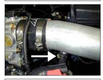
k. Attach the opposite end of the breather hose onto the nipple of the intake pipe. Secure it with a supplied 1" hose clamp.
