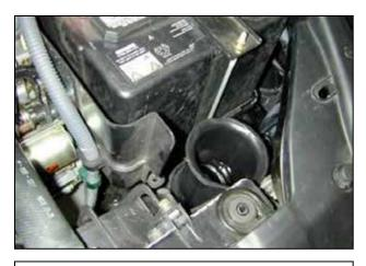
k. If equipped, remove the plastic air horn by pulling up.
