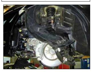
p. Partially remove the fender liner as shown.
