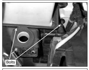
f. Loosen the two bolts holding the resonator box, and remove it.
