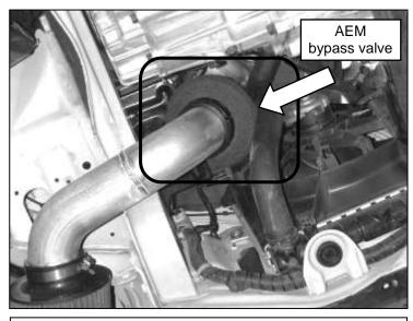
If an AEM<sup>®</sup> bypass valve (sold separately) is installed onto the AEM<sup>®</sup> intake system, install it in the location specified.
