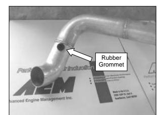
d. Install the factory rubber grommet removed from the air cleaner lid into the hole in the intake pipe.
