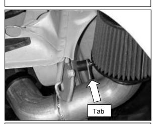
f. Using the included nut and washer, secure the tab of the intake pipe onto the rubber mount, as shown.
