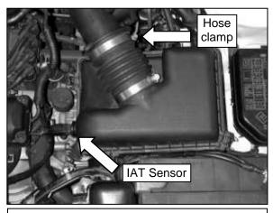
a. Unplug the Air Temp Sensor (ATS), loosen the hose clamp, unclip the air filter lid, and remove it. Remove the rubber ATS grommet and set it aside, as it will be used in the installation of the AEM<sup>®</sup> intake system.
