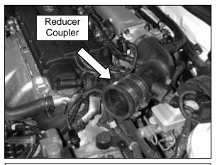
c. Install the included reducer coupler onto the MAF sensor, and secure it with the supplied No. 44 hose clamp.
