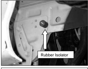
b. Install the included rubber isolator in the factory threaded hole in the frame rail, as shown.
