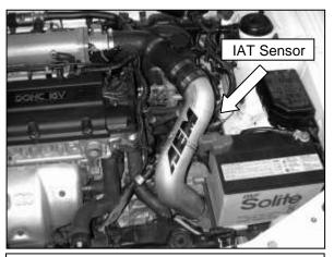
e. Install the intake pipe unto the reducer coupler, and insert the IAT Sensor into the rubber grommet, as shown. Loosen the battery hold down and move battery as close to the fender well as possible; then tighten the hold down clamps.
