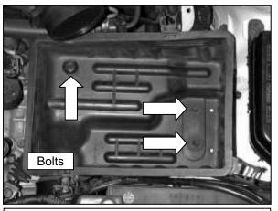
b. Loosen the three bolts holding the air cleaner base to the inner fender, and remove it.
