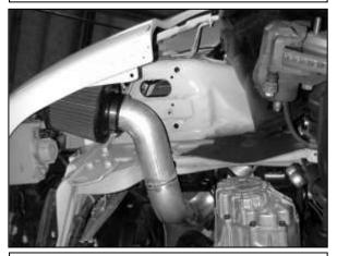
g. Install the air filter onto the intake pipe, and secure it with the supplied clamp.
