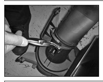
m. Using pliers, remove the stock hose clamp that is crimped onto the stock air filter box.
