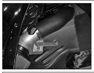
f. Place the intake system in the vehicle and align it as shown with the mounting bracket in place on the stud. Use one of the factory air filter box mounting nuts to secure the bracket. Don't tighten the nut at this point, but leave it loose enough to adjust the pipe.
