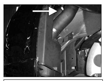
k. Remove the air filter box from the vehicle. It's helpful to guide the top hose out of the fender hole, and to pull the bumper slightly out for more clearance.
