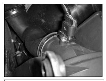
j. Reach to the top side of the air filter box and disconnect the MAF sensor harness.
