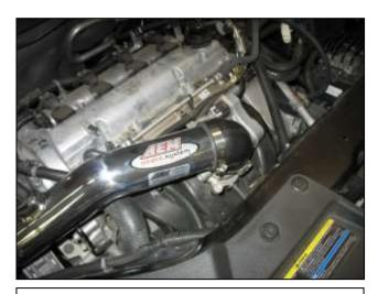
d. Assemble the intake pipe with the supplied 90 degree coupler and two #44 hose clamps. Line up the intake pipe bracket with the rubber mount. Then slide the coupler over onto the throttle body. Do not completely tighten the hose clamps or mounting hardware yet.
