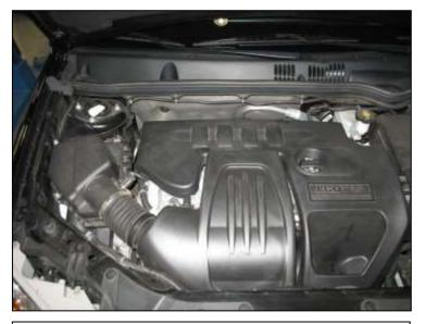
Factory air box system installed
