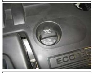
c. Remove the oil cap and then remove the engine cover. Re-install oil cap to avoid getting debris into your engine.
