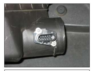
f. Remove the MAF sensor from the factory air box lid.
