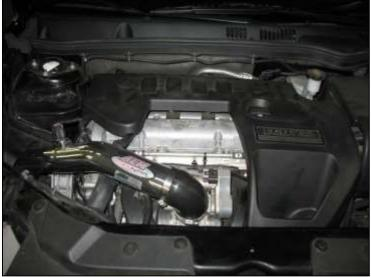
AEM® intake system installed
