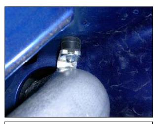
e. Use the supplied washer and serrated nut to secure the intake pipe. Install the air filter on the end of the pipe within the fender well. Secure the air filter to the intake pipe.
