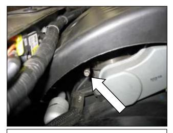
e. Loosen the hose clamp securing the stock inlet tube to the throttle body.
