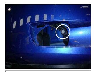
j. Remove the bolt at the front of the lower air box. Remove the lower air box from the vehicle. On the 2006 Cobalt you will need to gain access to this bolt by removing the front part of the fender liner and going underneath the car. After removing this bolt remove the lower box from the vehicle.
