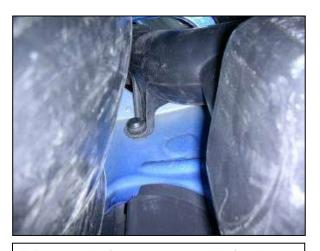
i. Remove the front passenger side fender liner to gain access to the lower air box. From inside the fender, release the plastic retainer near the top of the lower air box.
