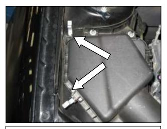
g. Release the two clips holding the air filter lid in place.
