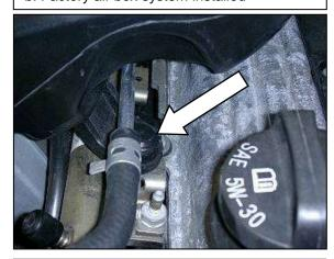
d. After removing the engine cover you will gain access to a plastic retainer near the fuel rail. Pry it open to being removal of stock air ducting.
