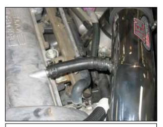
h. Secure the stock breather hose to the intake pipe nipple using the stock hose clamp.
