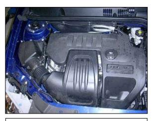
b. Factory air box system installed
