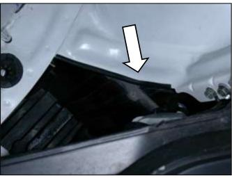
e. Install the rubber edge trim onto the metal lip behind the headlight.
