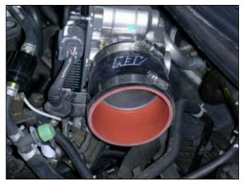
c. Slide the silicone coupler and supplied hose clamps onto the throttle body as shown.
