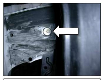
d. Install the rubber mount in the upper hole previously used to secure the lower air box.
