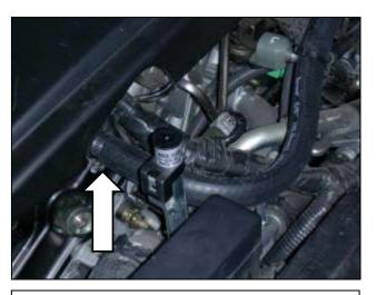
I. Secure one end of the supplied breather hose onto the valve cover with the supplied hose clamp.
