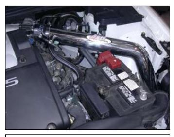
AEM® intake system installed
