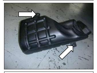
h. From inside the fender well, remove the two bolts that secure the lower air box. Then remove the lower air box from the vehicle.
