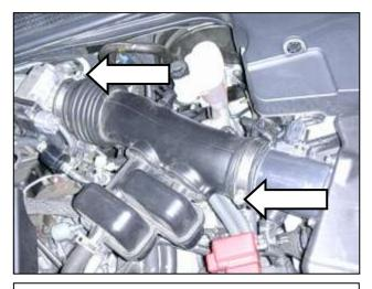
d. Loosen the two hose clamps on the ends of the inlet pipe. Remove the inlet pipe from the vehicle.
