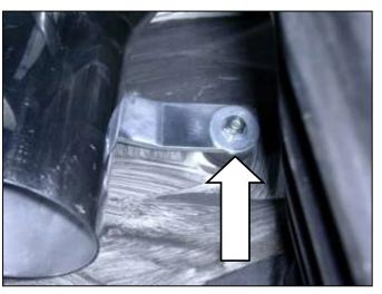
g. Place the large washer over the mounting tab. Lightly thread the lock nut over the washer.
