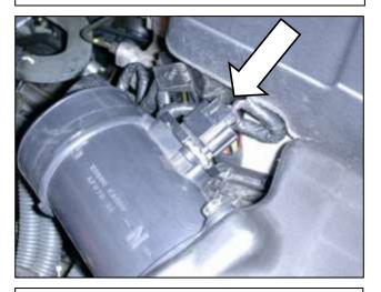
e. Free the clips that secure the mass air flow (MAF) sensor wiring harness. Unplug the MAF sensor.
