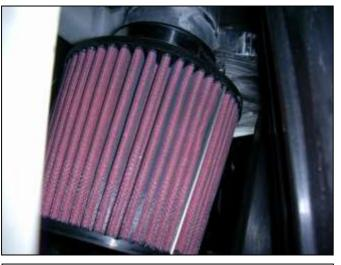
i. Place the air filter over the end of the inlet pipe. Tighten the air filter hose clamp.
