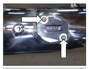
b. Utilizing the stock screws, install the MAF sensor into the  $\mathsf{AEM}^{\$}$  intake pipe.
