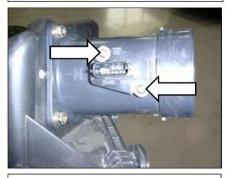
g. Loosen the screws that secure the MAF sensor. Carefully remove the MAF sensor.
