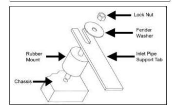
h. Proper installation of rubber mount assembly.
