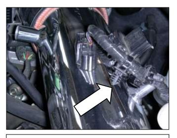
j. Attach the tree mount zip tie to the MAF sensor wiring harness. Trim the excess zip tie band.
