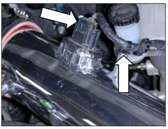
k. Plug the tree mount zip tie into the nipple near the MAF sensor. Plug in the MAF sensor.
