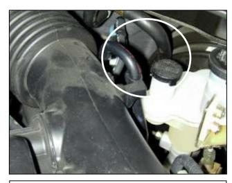
b. Free the differential breather hose from the inlet tube, if equipped. Use a supplied zip tie to secure the hose to the brake booster tube.
