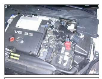
a. Stock air box system installed.
