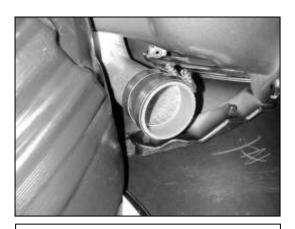
j. Attach the supplied coupler to the lower end of the upper intake pipe (located in the fender well). Loosely secure two of the provided hose clamps onto the coupler.
