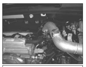
e. Install the upper intake pipe into the coupler on the throttle body. Leave the hose clamps loose for adjustment.
