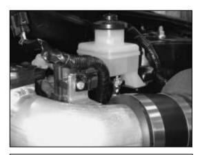
n. Plug in the MAF sensor wire harness connector back into the MAF sensor. Mount the EVAP VSV to the bracket on the upper intake pipe using the supplied M5 screw and washer. Insert the screw through the wire harness clip and through the intake pipe bracket so it threads into the VSV. Adjust the wires so that they are not in tension.
