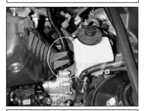
i. Free the wire harness loom clip by gently squeezing the sides in. Remove the lower airbox from the engine bay.
