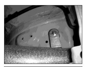
g. Loosely secure the second bracket to the rubber mount with a washer and nut.
