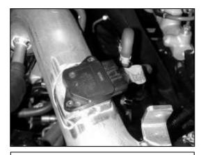
m. Secure the MAF sensor to the AEM<sup>®</sup> intake pipe with the supplied 8-32 bolts. Use care to avoid damaging the o-ring.
