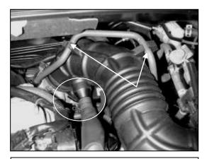
b. Pull the EVAP purge hose free from the two rubber clips on the intake hose. Remove the crankcase breather hose from the intake tube. Save the factory clamp for use later in the installation.
