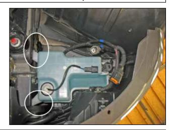
h. Remove two M6 bolts securing the washer bottle. Unplug the hose from the washer pump and remove the washer bottle from the car. Drain any remaining washer fluid into a clean container so it can be reused.
