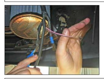
n. If the vehicle is equipped with fog lights, unwrap the wire loom as shown and separate the fog light wires.
