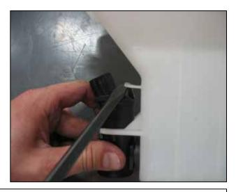
j. Using a flat head screwdriver, unclip the washer pump from the washer bottle as shown.
