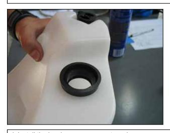
d. Install the level sensor grommet as shown.
