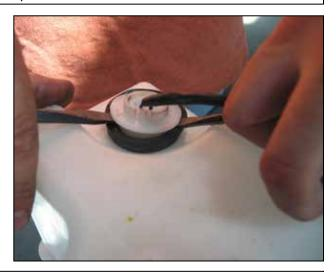
I. Using two flat head screwdrivers, carefully pry up on the lip of the washer level sensor. Take care not to damage the rubber grommet. Some liquid soap and water mixture applied to the sensor may help with removal. Also remove the grommet and set it aside.
