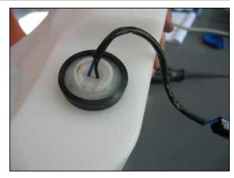
e. Apply liquid soap solution to the level sensor and insert it into the grommet. Make sure that the level sensor is pressed all the way into the grommet. The lip of the sensor should be inside the grove of the grommet.
