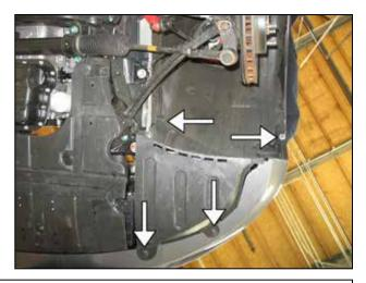
f. Lift the car and remove the right front wheel. From underneath the vehicle, remove three clips and one screw from the inner wheel well liner. Pull the wheel well liner back out of the way.
