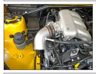
h. Install the upper pipe and 3.5" x 2" throttle body coupler as shown with two #60 Clamps. Secure the crankcase vent hose to the nipple on the inlet pipe with the OE spring clamp. Plug in the headlight unplugged in Step 2e.
