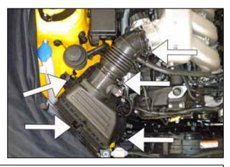
b. Unclip the four airbox clips and loosen the clamp at the throttle body. Unplug the MAF sensor.
