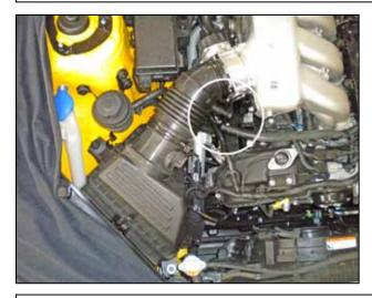
c. Unhook the crankcase vent hose by sliding back the spring clamp, then pulling the hose off of the nipple on the inlet tube. Remove the airbox lid and stock inlet tube assembly.
