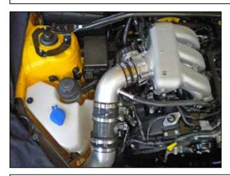
p. Plug in the washer pump and washer fluid level sensor. Reattach the washer fluid hose to the pump and fill up the washer bottle, then snap on the blue washer fluid cap.
