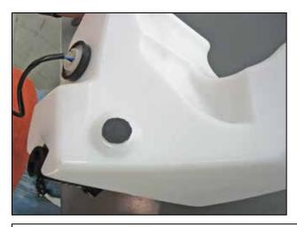
f. Apply the self adhesive rubber pad onto the protrusion on the underside of the washer bottle as shown. Set the new washer bottle assembly aside.
