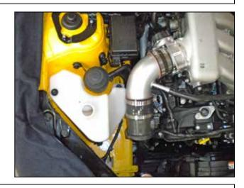
k. Install the washer bottle assembly and attach it with two of the M6 bolts removed in step 2d.
