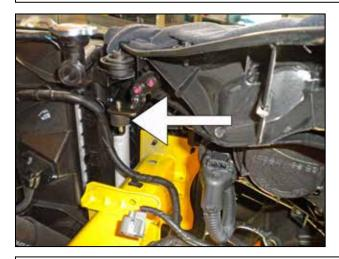
j. Install the supplied M6 rubber mount from the underside of the bracket as shown.
