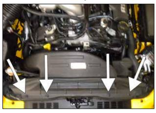
a. Remove four clips and remove air duct.
