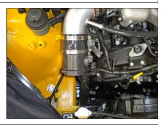
i. Attach the MAF sensor to the upper pipe as shown using the 3.5" x 3" coupler and two #60 clamps. Be sure that the MAF sensor is oriented as shown, and arrow on the MAF is pointing toward the engine.
