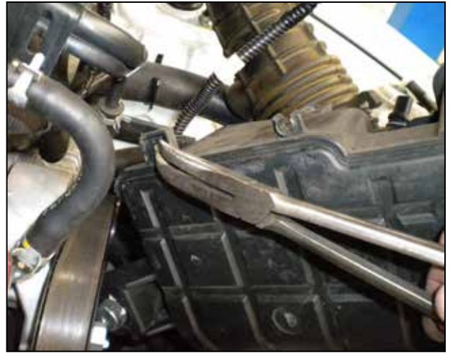
l. Disconnect the second zip tie securing the IAT harness to the air box; then remove the air box.
