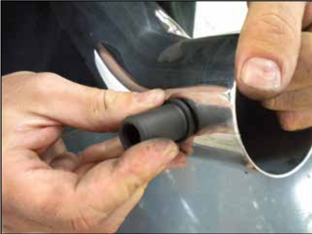
b. Install the PCV adapter in the upper pipe.
