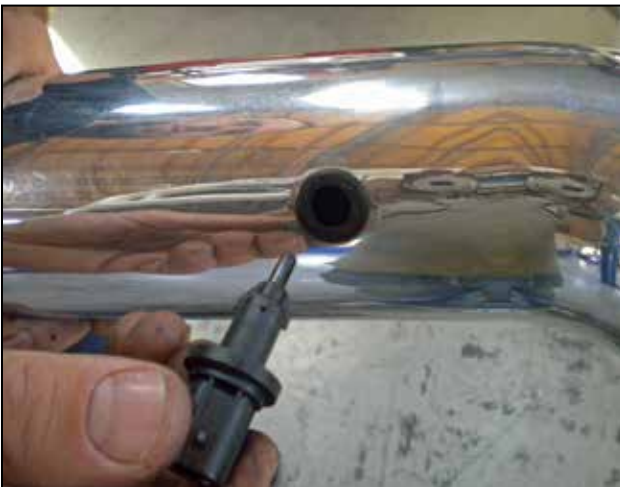
f. Install the IAT sensor into the middle pipe.
