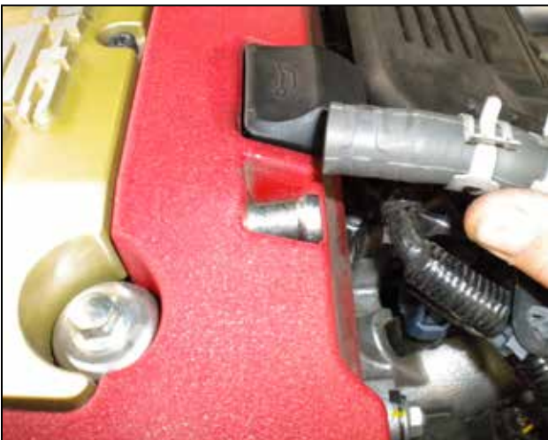
i. Disconnect the PCV hose connected to the valve cover port.
