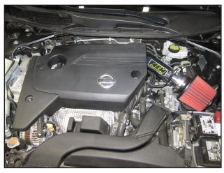
Make sure all the hose clamps and fasteners are tight then install the engine cover.
