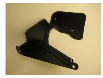
a) Install the upper edge trim (8-3034) onto the top of the heat shield. Then install the lower edge trim (102488) onto the bottom of the heat shield as shown. **Note: Cut edge trim to fit.**
