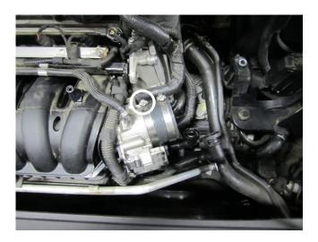
c) Install the hose and hose clamps onto the throttle body. Tighten the hose clamp closest to the throttle body at this time.
