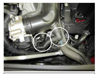
d) Detach both of the air injection connectors by squeezing the knurled area and pulling away from the stock intake tube. **Note: Some models have only one vent.**
