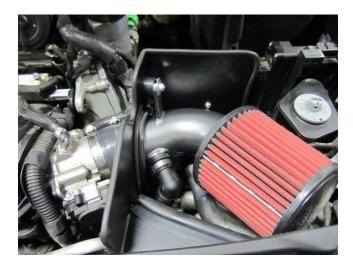
j) Install and tighten the air filter and hose clamp (9452) onto the AEM intake tube. Note: Rotate the filter for best clearance, so it does not make contact with anything in the engine compartment.
