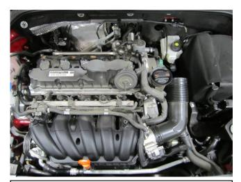
c) Remove the engine cover from the vehicle. Note: Pull up on the back corners of the cover first then the front two.
