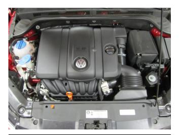
Factory air box system installed
