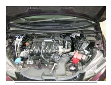
p. Finished installation of AEM Intake System.
