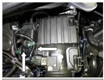
c. Disconnect the MAF harness from the connector. Unclip the two green tree-mount ties from upper airbox.
