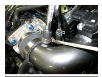
h. Connect the breather line to the intake tube using the hose(AEM-5-1002) and fasten hose clamp(AEM-4093-5). The hose may need top be trimmed for proper fitment.
