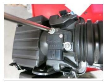
f. Use a phillips screwdriver to remove the MAF sensor. Set aside the stock screws for use with the AEM tube.
