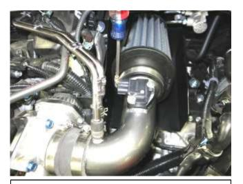
k. Align the filter vertically and tighten the hose clamp to secure its position.
