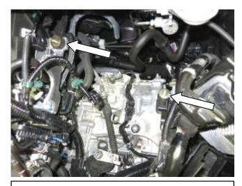
c. Install the two rubber mounts(AEM-1228598) onto the stock airbox mounting locations as indicated.
