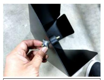
d. Install the rubber mount(AEM-1228599) onto the heat shield(20-8545) as shown and fasten with the provided washer(08160) and nut(AEM-460.04).
