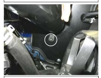
h. align the AEM intake bracket with the rubber mount.
