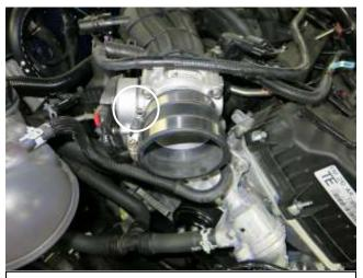
f. Install the coupler onto the throttle body with the provided hose clamps and tighten the one closest to the throttle body.
