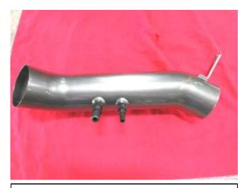
a. Install the two provided vent adapters into the tube as shown. Manual transmissions will use the plug provided instead of the vent adapter on the right side. Install finger tight, then a 1/4 turn with a wrench.
