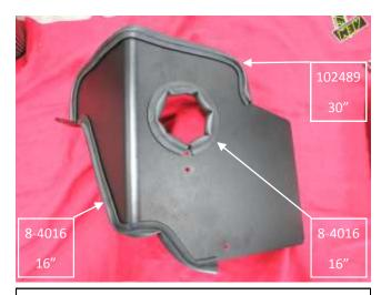
b. Install the provided edge trims onto the heat shield.
