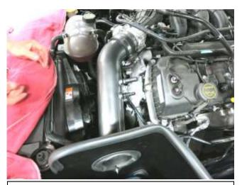
g. Install the AEM intake tube into the coupler and the heat shield opening.
