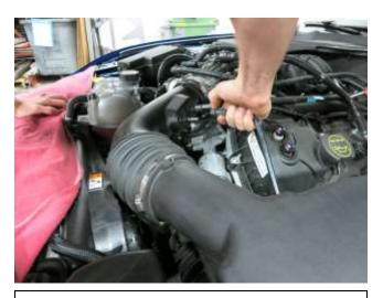
d. On automatic transmissions depress the gray clip and pull the second vent line from the stock intake. Manual transmissions will not have this vent line. Then remove the stock intake and air box from the vehicle.
