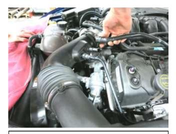
c. Unlatch the gray clip on the connector and pull the vent line from the stock intake tube.
