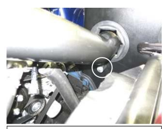
i. Install the provided bolt and washer and tighten the AEM intake tube bracket to the rubber mount.
