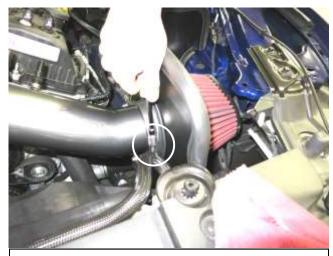
$\ensuremath{k}.$  Slide the hose clamp over the filter and tighten at this time.
