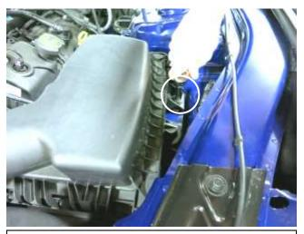
b. Remove the bolt securing the air box to the vehicle. This will be reused in step 3d.
