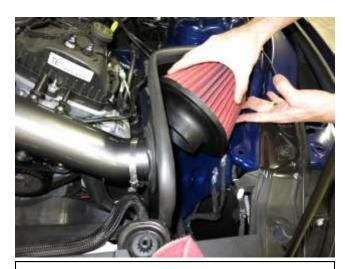
j. Install the hose clamp over the AEM intake tube and slide the AEM filter onto the tube as shown.
