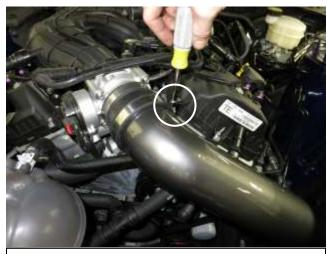
I. Tighten the other hose clamp furthest from the throttle body at this time.
