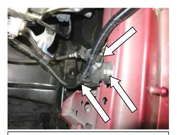
h. Use a flathead screwdriver to release the clutch cable from the plastic clip. Remove the M6 bolt securing the metal bracket. Detach the tree mount zip tie from the bracket and set the bracket aside.
