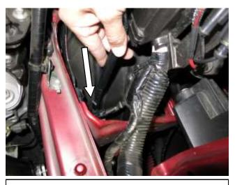
f. Route the MAF harness down along the fender wheel liner as shown.
