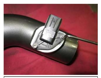
a. Install the MAF sensor from step 2g into the AEM tube and secure it using the M4 bolts(07733) provided.
