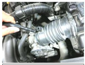
c. Disconnect crank case breather hose from stock intake tube.
