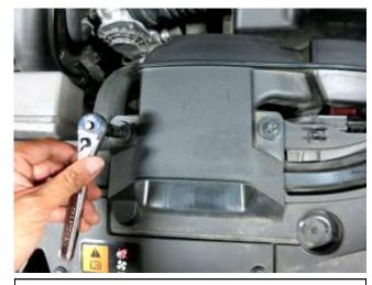
e. Remove the two M6 bolts securing the intake inlet air duct.
