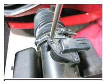
g. Loosen the two screws using a phillips screwdriver and set MAF sensor aside.
