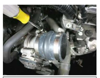
b. Install the hump hose(AEM-5-575) onto the throttle along with two hose clamps(AEM-9444). Only tighten the hose clamp on the throttle at this time.
