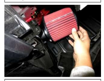
i. Lower the flap of the fender liner to install the AEM filter(AEM-21-202DOS) and hose clamp(AEM-9444) onto the intake tube. Connect the harness to the MAF sensor.
