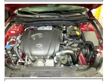
n. Finished installation of AEM Intake System.
