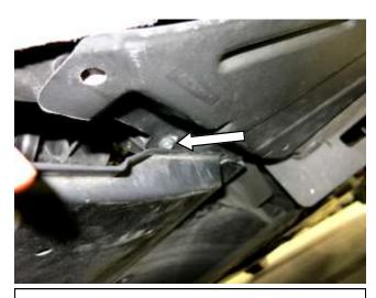
h. Pull down on the large plastic cover to access the bolt indicated. Remove the bolt using an 8mm socket.
