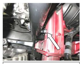
e. Loosely fasten the mounting bracket using the provided washer (08160) and bolt from step 2h.
