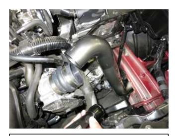
c. Position the AEM tube as shown to allow the lower end to slide into the wheel well location.
