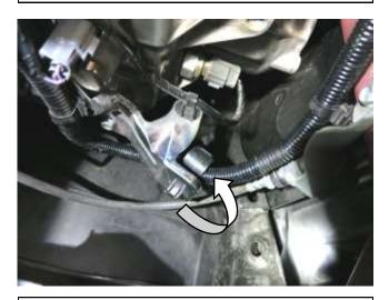
i. Release the clutch cable from the lower plastic clip. Remove the clip and reinstall it on the backside of the original location as shown. Re-fasten the clutch cable to the clip in the new location .
