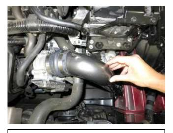
d. Rotate the tube towards the radiator and carefully slide the tube into the hump hose.
