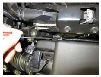
a. Disconnect MAF harness from sensor. Use a flathead screwdriver to detach tree mount clip from air box lid.
