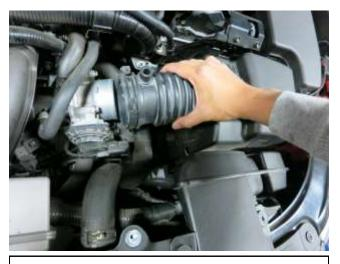
f. Detach the intake tube from the throttle and carefully remove the stock intake assembly from the engine bay.
