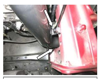
j. Adjust tube position to achieve clearance and tighten M6 bolt. Rotate the filter to clear the fender liner and tighten the hose clamp .
