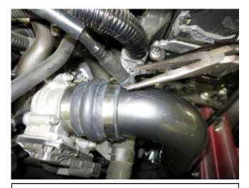
k. Trim 3/4 inch off the provided hose(AEM-5-1002) and install it onto the intake tube along with the spring clamp (08552). Connect the plastic hard line to the hose.
