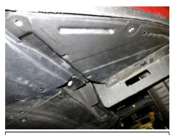
I. Reinstall the lower plastic covers and secure with previously removed hardware. Check final clearance and tighten the hose clamp on the hump hose.
