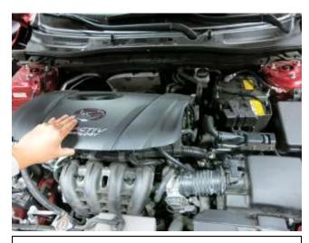
b. Remove engine cover by pulling up towards hood as shown.
