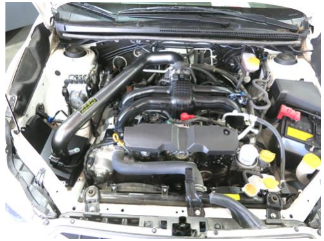
AEM INTAKE INSTALLED
