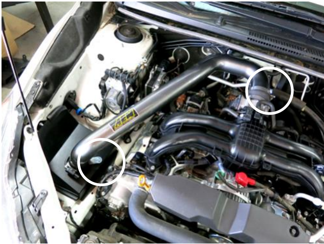
f. Install the AEM intake tube into the vehicle aligning it with the coupler and the hole in the heat shield. Using the provided hardware, secure the bracket to the heat shield. Tighten the hose clamp at this time.
