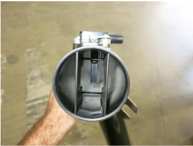
e. Install the MAF insert into the end of the tube and align it as shown. Note: Use a few drips of super glue on the insert's lip to hold it in place in the tube.
