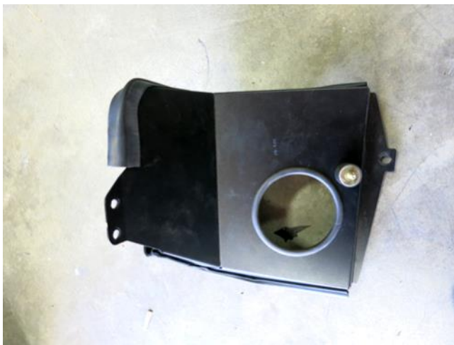
a. Install the edge trim and rubber mount onto the AEM heat shield according to the parts diagram on pg. 2.
