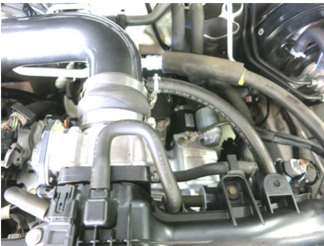
i. Install the new provided vent hose from the AEM intake tube to the engine where step 2g was disconnected. Secure with the factory spring clamps removed in step 2g.
