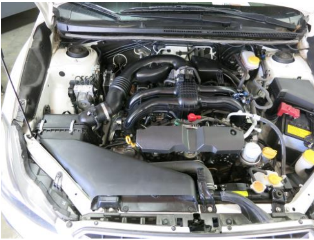
STOCK INTAKE INSTALLED
