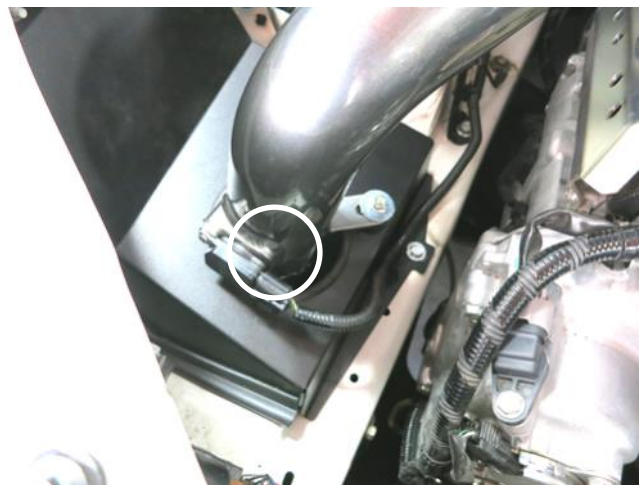
j. Plug the mass air sensor connector back into the mass air sensor.
