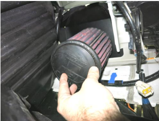
g. Install the AEM filter onto the AEM intake tube from under the vehicle and secure with the provide hose clamp.
