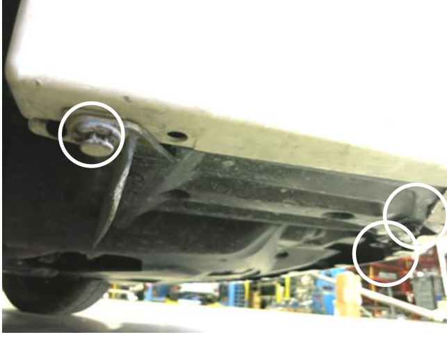
h. Reinstall the 3 clips and secure the passenger side lower splash shield to the bumper.
