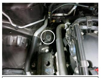
d. Remove the rubber grommet from the vehicle. This will not be reused.
