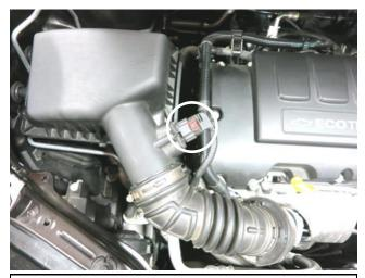
a. Release the red tab on the mass air sensor connector and disconnect the connector from the sensor.
