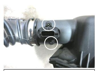
f. Remove the two screws securing the mass air sensor to the stock upper air box. The screws will not be reused, however the mass air sensor will be reused in step 3g.
