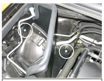
d. Install the completed AEM heat shield into the vehicle aligning the mount on the inner fender and rear rubber grommet.
