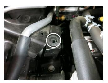
a. Take the rubber grommet that was removed in step 2e. and install it into the same location the rubber grommet in step 2d. was removed.
