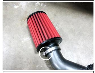
h. Install the AEM filter onto the AEM intake tube and secure with the provided hose clamp.
