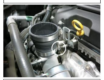
f. Install the coupler and provided hose clamps on to the turbo compressor inlet. Tighten the hose clamp closest to the compressor at this time.
