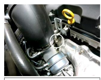
b. Loosen the hose clamp at the turbo compressor inlet.
