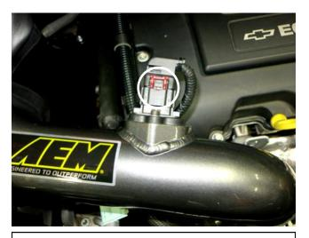
j. Reconnect the mass air sensor connector onto the mass air sensor. Engage the red locking tab.
