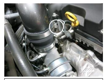
Install the AEM intake tube into the vehicle aligning the tube with the coupler. Tighten the hose clamp (circled above) at this time.
