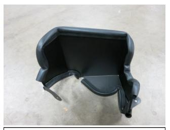
b. Install the edge trim onto the AEM heat shield as shown, trim to fit if desired.
