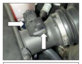
b. Unplug the wire harness from the Mass Air Flow (MAF) sensor. Remove the two screws securing the MAF sensor, then carefully remove the MAF sensor and set aside.
