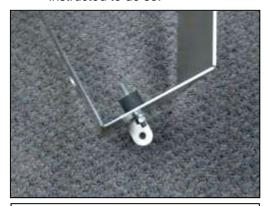
b. Install the supplied rubber mount onto the AEM® heat shield using a washer and locknut as shown.
