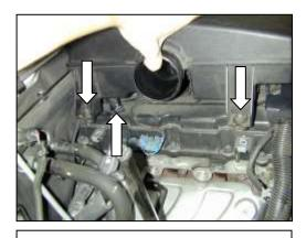
e. Remove the two bolts securing the resonator onto the valve cover. Lift the resonator up, then remove the breather hose from the valve cover and remove the resonator.
