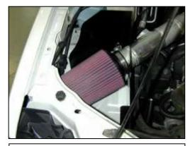
k. Tighten the hose clamps at the throttle body. Tighten the nut on the mounting bracket. Re-adjust the intake pipe if necessary. Plug the MAF sensor harness into the sensor.
