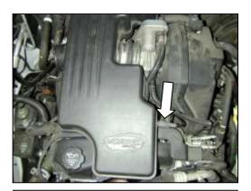
d. Loosen the hose clamp securing the intake resonator to the throttle body.
