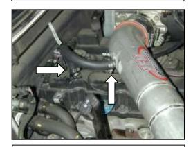
i. Attach the supplied ½" hose between the intake pipe and the valve cover inlet as shown. Trim to fit and secure using the supplied hose clamps.
