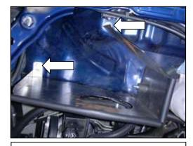
c. Install the AEM® heat shield, using two supplied bolts and washers and the stock mounting nut removed in step 2c. Install rubber edge trim to the top edge of the heat shield
