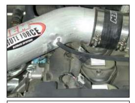
j. Attach the supplied 3/16" vacuum hose between the hard plastic breather hose and the intake pipe.
