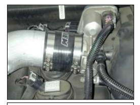
f. Slide the bracket side of the intake pipe through the heat shield hole. Insert the nipple side of the intake pipe into the 3" silicone hose on the throttle body.
