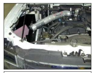
AEM® intake system installed
