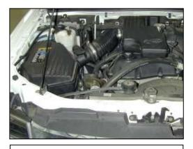
a. Factory airbox system installed.
