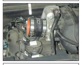
e. Install the 3" silicone hose onto the throttle body; secure using the #48 hose clamp. Install the remaining #48 hose clamp onto the opposite end.
