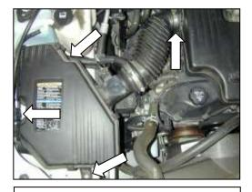
c. Loosen the hose clamp securing the airbox assembly to the intake resonator. Remove the nut and two bolts securing the airbox, lift the airbox up and out of the vehicle.
