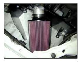
h. Ensure the AEM<sup>®</sup> air filter is clear of debris. Attach the air filter onto the end of the AEM<sup>®</sup> intake pipe and secure with a hose clamp as shown.
