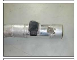
d. Install the MAF sensor using the stock mounting screws. Use caution to avoid damaging the o-ring.
