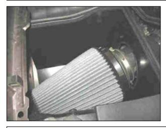
i. Install air filter assembly into the stock MAF rubber coupler.
