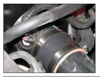
g. Then attach the assembly made in step 3g. to the end of the intake pipe. Reconnect the MAF sensor wire.
