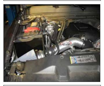
AEM<sup>®</sup> intake system installed
