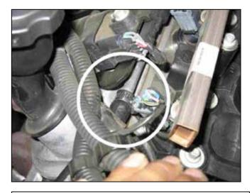
I. Secure the supplied breather hose with the supplied hose clamp.
