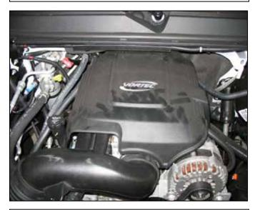
Factory air box system installed
