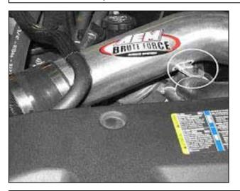
j. Use the stock plastic radiator clamp to secure the radiator hose away from the intake pipe. By inserting it into the bracket located on the pipe.
