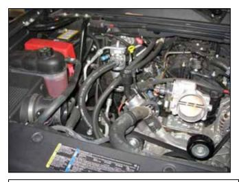
f. Pull the stock inlet tube out of the vehicle. Loosen the hose clamp securing the MAF housing to the air filter, remove MAF housing, keep for later reuse.
