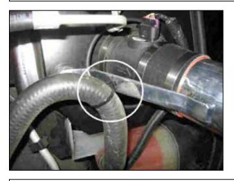
n. Insert tree mount into intake pipe bracket, secure radiator overflow hose to tree mount.
