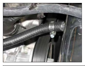
m. Secure the breather hose to the nipple on the intake pipe.
