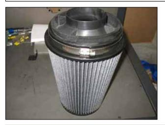
h. Create the air filter assembly by inserting the air filter adapter into the air filter as shown. Once in place secure the hose clamp.
