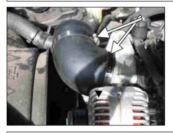
d. Install the elbow onto the throttle body, and loosely put the supplied hose clamps on the ends.
