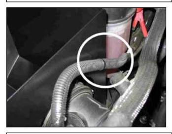
k. Use the supplied tree mount to secure the MAF sensor wire to heatsheild.
