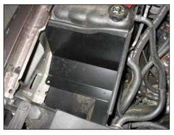
c. Install the heat shield using the three stock bolts used to secure the air filter box mounting plate.
