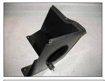
b. On the heat shield, install rubber mount using the supplied washer and nut. Install "8-3018" rubber edge trim around intake pipe opening. Install 8-4011 and 8-4012 edge trim to top edge of the heat sheild.
