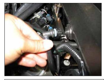
b. Pull out the breather hose out of the resonating chamber in the stock air box system.
