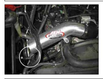
e. Insert intake pipe into elbow located at the throttle body. Secure the bracket to the rubber mount on the heatshield.
