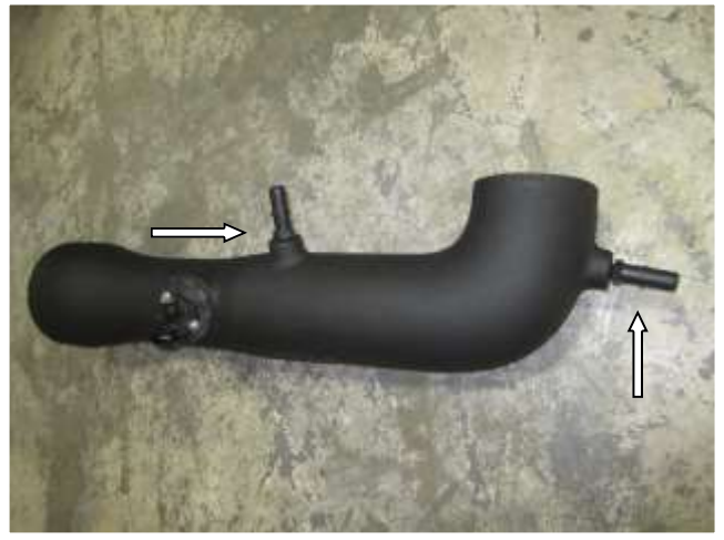
d. Install the two vent hose fittings into the tube. Note: Hand tighten, then add a quarter turn with a wrench.
