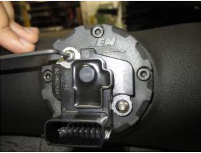
c. Install the mass air sensor into the mass air sensor adapter that has already been attached to the AEM intake tube with the provided M4 allen's. Note: Be very careful with the mass air sensor.
