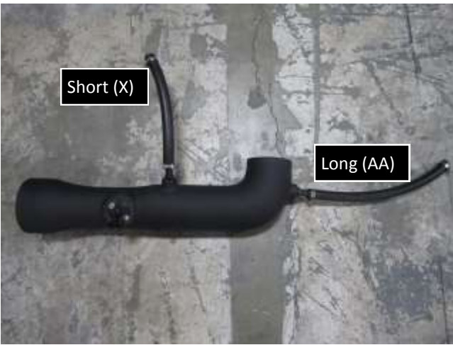
e. Slide the two supplied vent hoses and four clamps onto the vent fittings and tighten. The shorter hose will go on the left vent, and the longer hose will go on the right vent.
