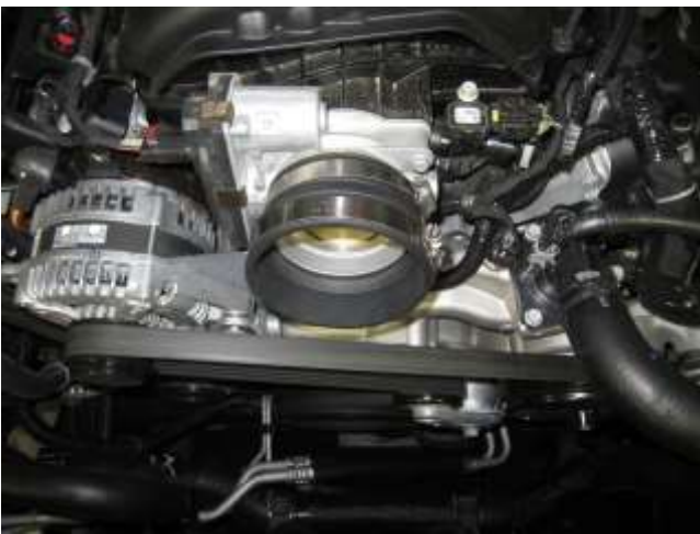
g. g. Install the throttle body coupler with hose clamps 5.3L use p/n 341018 and #56; 6.2L use p/n 341014 and #64. Do not tighten clamps at this point.
