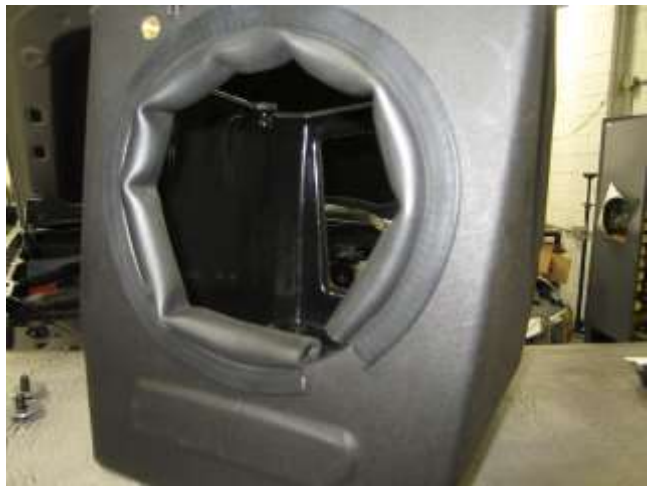
f. Install the edge trim onto the AEM air box, trim off excess if necessary.
