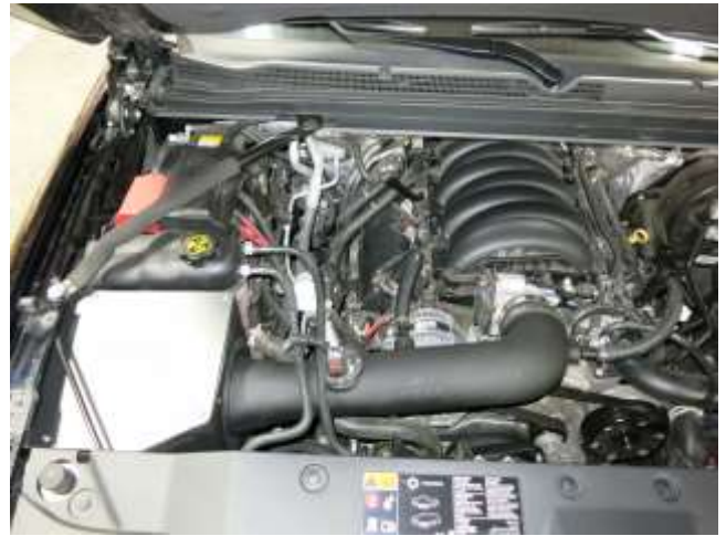
AEM intake system installed
