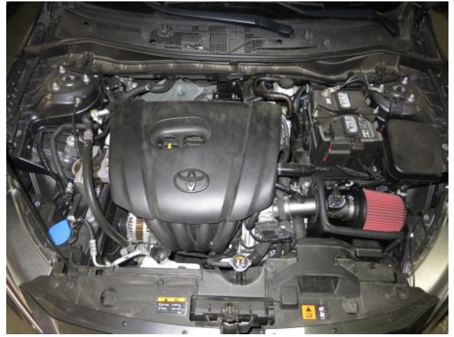
AEM INTAKE INSTALLED
