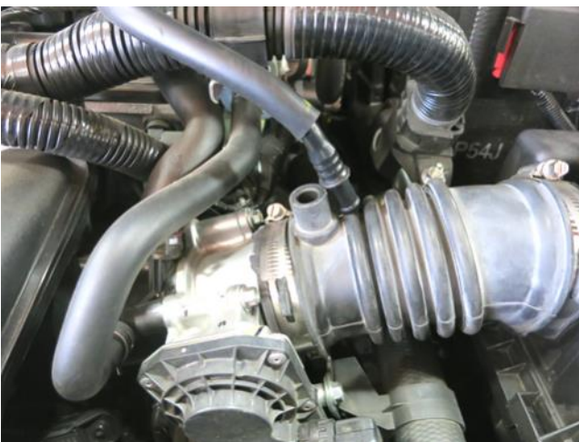
c. Use a 7mm socket and ratchet to loosen the throttle body hose clamp. Then, pull the PCV line out from the nipple on the intake hose.
