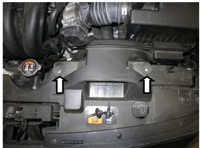
d. Use a 10mm socket and ratchet to remove the (2) M6 bolts holding the intake snorkel to the radiator shroud. These bolts will be reused in step 3f.
