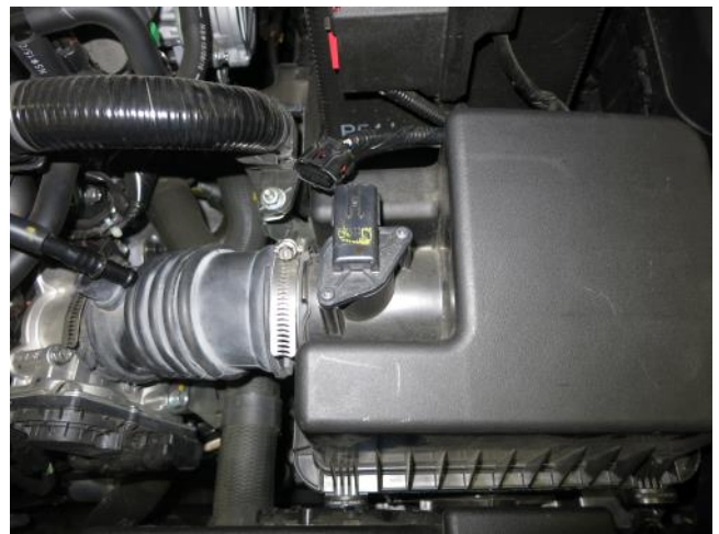
b. Unplug harness from MAF (Mass Air Flow) sensor.
