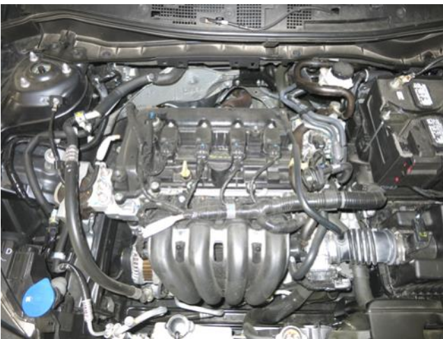
a. Carefully pull up on the engine cover and remove it.
