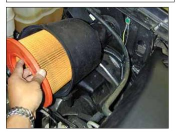
i. Remove filter element and housing. Gently pull up on the housing to remove.
