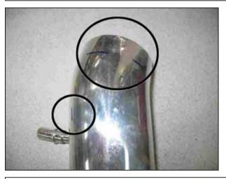
k. Mark a line 1" from the end of the inlet tube and 2" from the nipple, on the outside of the bend.
