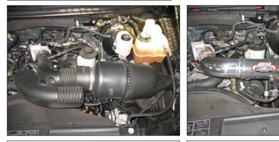
Factory air box system installed
