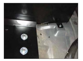
h. Secure the rest of the heatshield with the two supplied lock nuts and washers.
