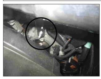
s. Loosely secure the bottom bracket with the 559960 washer and 444.460.08 nut.
