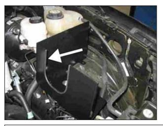
i. Install the rubber edge trim on the pipe opening on the heatshield.
