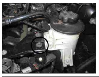
o. Remove the front bolt from steering pump fluid reservoir bracket.
