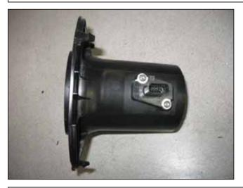
h. Remove the mass airflow sensor from the air box using the supplied torx tool (Be sure to keep the sensor in a safe place to be used later).
