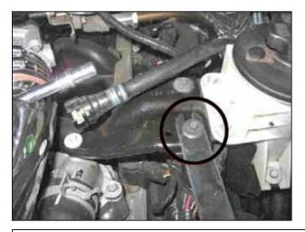
t. Loosely secure the top bracket with the bolt removed in 30.
