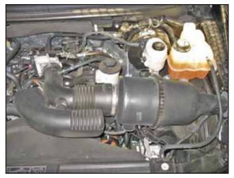
a. Factory air box system installed.
