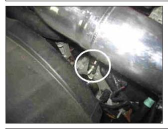
q. Align the bottom bracket over the stud protruding from the left hand cylinder head.
