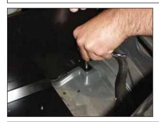
g. Place the heatshield in the engine bay and screw in the supplied self tapping screw.
