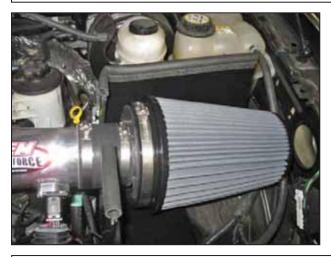
w. From inside the heat shield, slide the filter assembly over the inlet pipe and loosely secure with #56 hose clamp.
