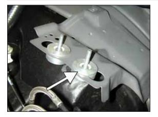
d. Insert the assembly from Step 3c. into the upper spacer from underneath. Secure with provided nut.
