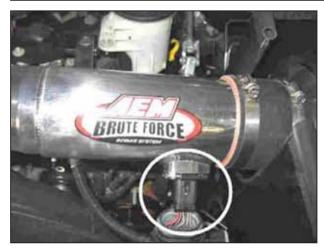
y. Reconnect the mass airflow sensor harness to the mass airflow sensor and lock it.
