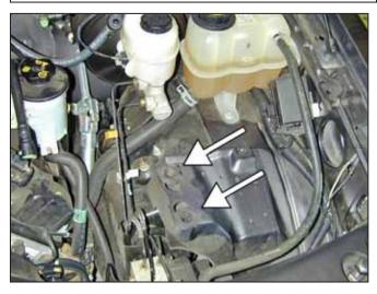
j. Remove rubber grommets left by the filter element housing.
