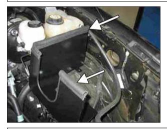
j. Install the rubber gasket on the top edges of the heat shield.
