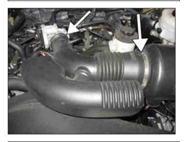
c. Loosen hose clamps at the throttle body and the air filter housing.
