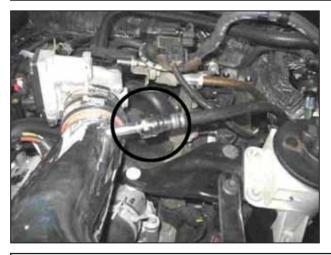
x. Connect the breather hose to the to the inlet pipe.
