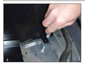
e. Place the heathshield into the engine bay aligning the two holes located on the bottom face of the heat shield with the two bolts installed in step 3d. With a marker, mark the location of the thrid hole.
