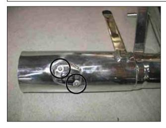
m. Install the mass airflow sensor into the straight section of the inlet pipe. Use the two factory torx bolts to secure the sensor.
