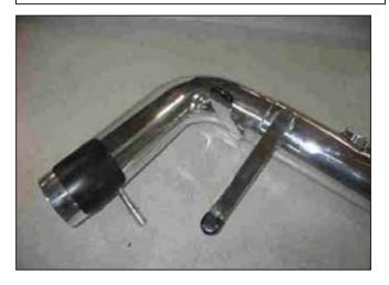
I. Apply rubber patch from the line marked in 3k. on the outside of the bend. Make sure to place the patch on the underside of the tube.
