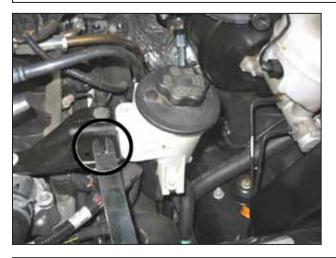
r. Align the top bracket over the threaded hole in the steering pump fluid reservoir bracket.
