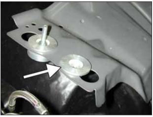
c. On the left is a fully assembled anchor for the heat shield. On the right, insert the upper spacer into the stock housing mounting surface.
