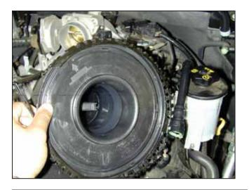
f. Gently pry open the housing at the any one of the tabs. Be careful not to damage the MAF sensor.
