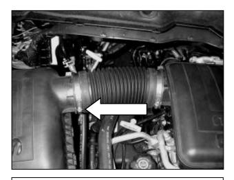
a. Loosen the hose clamp at the air box. Pull the rubber air hose away from the air box lid.
