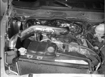
AEM® intake system installed
