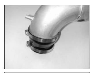
j. Loosely install the coupler and hose clamps on to the end of the  $\mathsf{AEM}^{\$}$  inlet pipe nearest the vacuum nipple.
