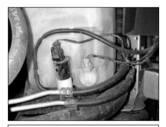
b. Unplug the wire connectors going to the windshield washer fluid pump and level indicator. Unplug the washer fluid hose. Block the nipple on the pump to prevent the washer fluid from draining.
