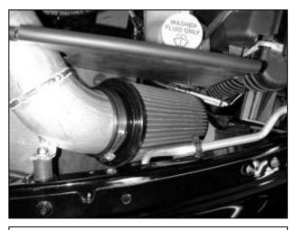
n. Install the AEM<sup>®</sup> air filter from inside the fender well. Slide the air filter on to the pipe until it stops. Secure with the supplied hose clamp. Make sure the windshield washer wires and hose do not come into contact with the air filter.
