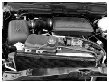
Factory air box system installed
