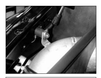
k. Install the bracket end of the AEM® inlet pipe through the cutout in the heat shield. Install the coupler on to the throttle body. The bracket will line up with the rubber mount installed in step 3b. Loosely secure the bracket with the supplied washer and locknut. Refer to the diagram below for proper rubber mount installation.
