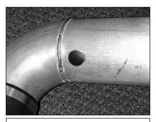
h. On 2002 models install the supplied polyethylene plug into the hole in the  $\mathsf{AEM}^{\otimes}$  inlet pipe.
