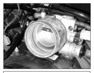
i. Remove the rubber adapter from the throttle body.
