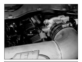
I. Reconnect the wire harness to the IAT sensor (if applicable). Do not push the grommet through into the pipe.
