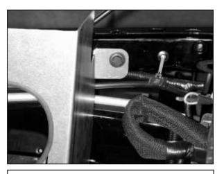
g. The rear mounting tab on the heat shield will line up with one of the lower air box mounting holes. Install one of the original bolts. Adjust the heat shield for best fitment then tighten the three mounting bolts.
